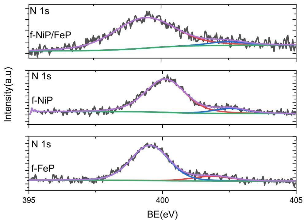
**Figure S4.** High-resolution XPS spectra of N 1s for f-FeP, f-NiP, and f-NiFeP.
