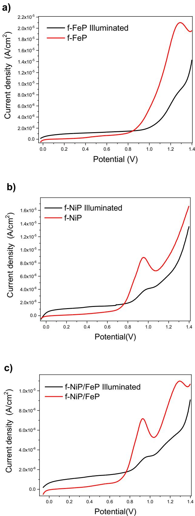
**Figure S6.** LSV with and without illumination with Xenon lamp, for a) f-FeP, b) f-NiP, and c) f-NiP/FeP (potential vs RHE).
