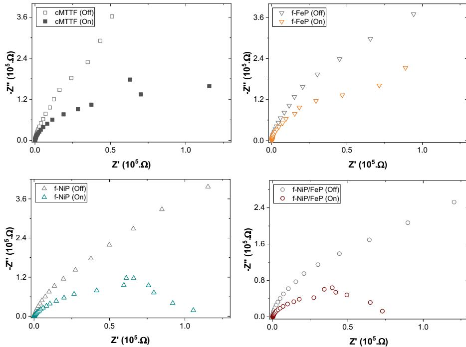
**Figure S7.** Nyquist diagrams of bare cMTTF, f-FeP, f-NiP, and f-NiP/FeP with (On) and without (Off) light.
