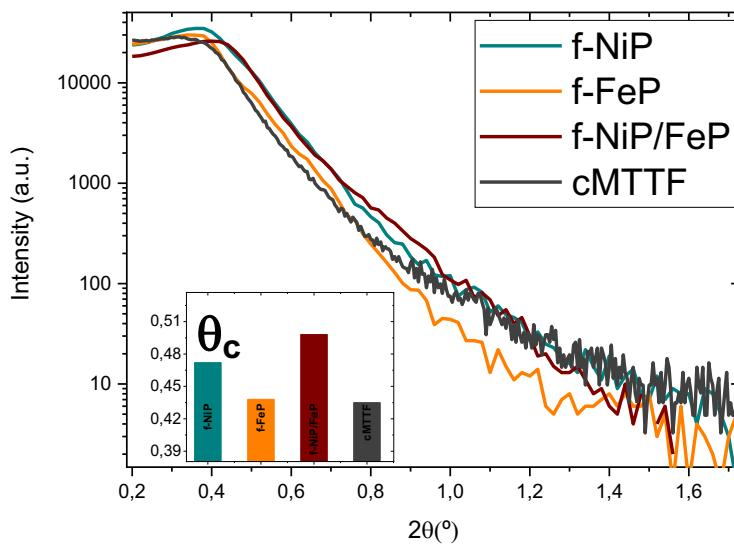
**Figure S3.** XRR patterns showing the critical angle region for cMTTF, f-NiP, f-FeP, and f-NiP/FeP.
