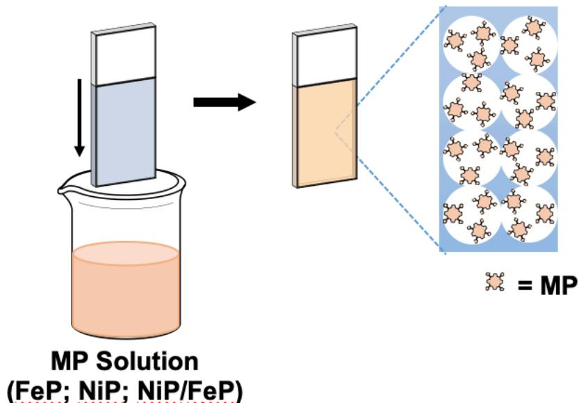
**Scheme S1.** Synthetic procedure for f-FeP, f-NiP and f-NiP/FeP.
