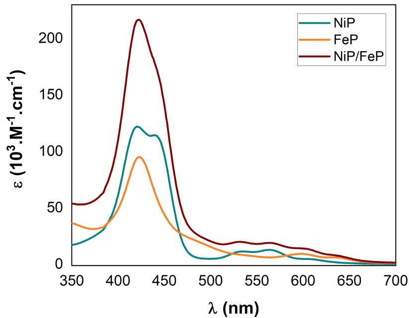
**Figure S2.** Molar extinction coefficient spectra of FeP, NiP, and NiP/FeP in water.
