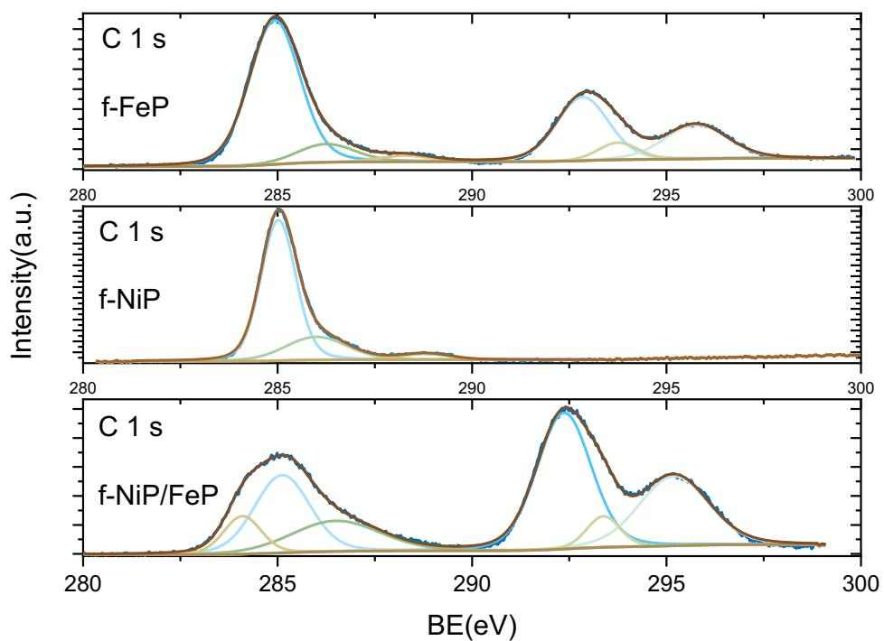
**Figure S5.** High-resolution XPS spectra of C 1s for f-FeP, f-NiP, and f-NiFeP.
