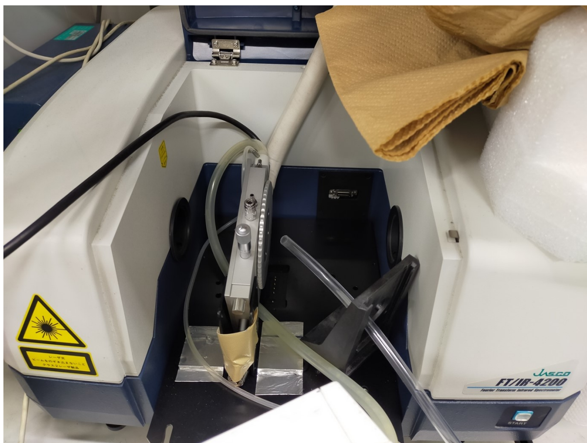
Fig. S1 Photograph of the thermally controlled FTIR spectroscopic system.
