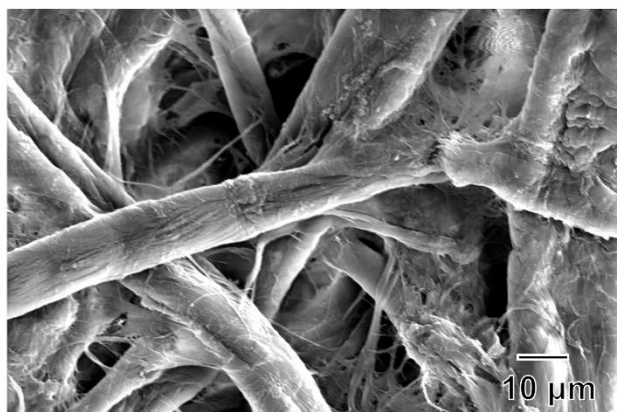
Fig. S12 FE-SEM image of the 1_{\text{Poly}} -printed PCSAD after adding \text{Cu}^{2+} ions ( 3.0 \times 10^{-3} M).
