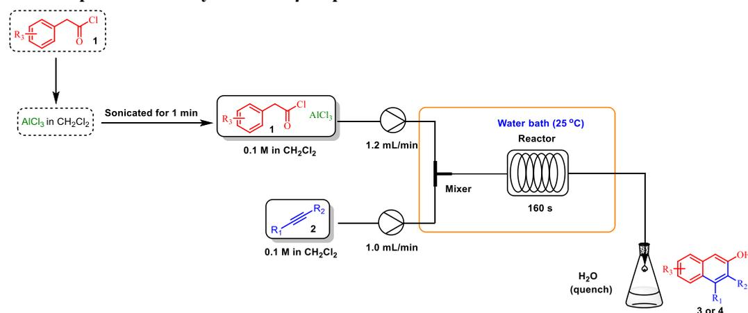
Fig. S1 The flow system for the synthesis of  $\beta$ -naphthols.
