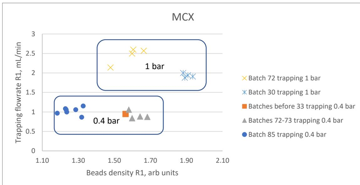
**Figure 1.** Distribution of cassettes batches as function of their bead's density and trapping flowrate in R1 chamber: top image – cassettes with R1 filled with PS-H+ resin; bottom image – cassettes with R1 filled with MCX beads.
