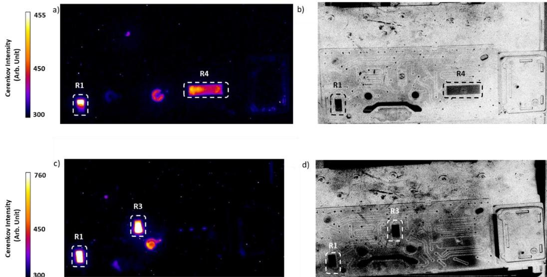
**Figure 3.** Cerenkov and white light images obtained after the  $[^{68}\text{Ga}]\text{Ga-PSMA-11}$  production using the cassette with formulation in R4 (a, b) and in R3 (c, d) chambers.
