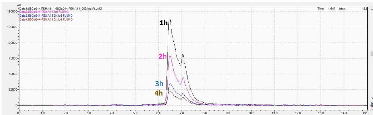
**Figure 4.** Overlaid radiochromatograms of [<sup>68</sup>Ga]Ga-PSMA-11, demonstrating its stability within 4 h from the final product delivery.
