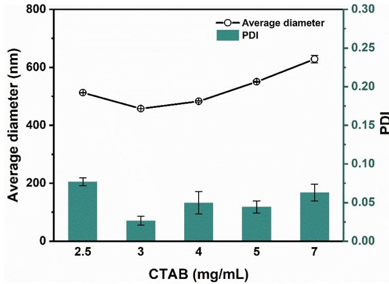
**Fig. S3.** Effect of CTAB concentration on the average particle size and PDI value\_of the HMONS.
