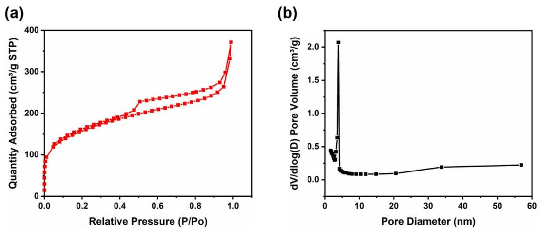
**Fig. S2.** (a) Nitrogen adsorption/desorption isotherms, (b) mesopore size distribution of the HMONs.
