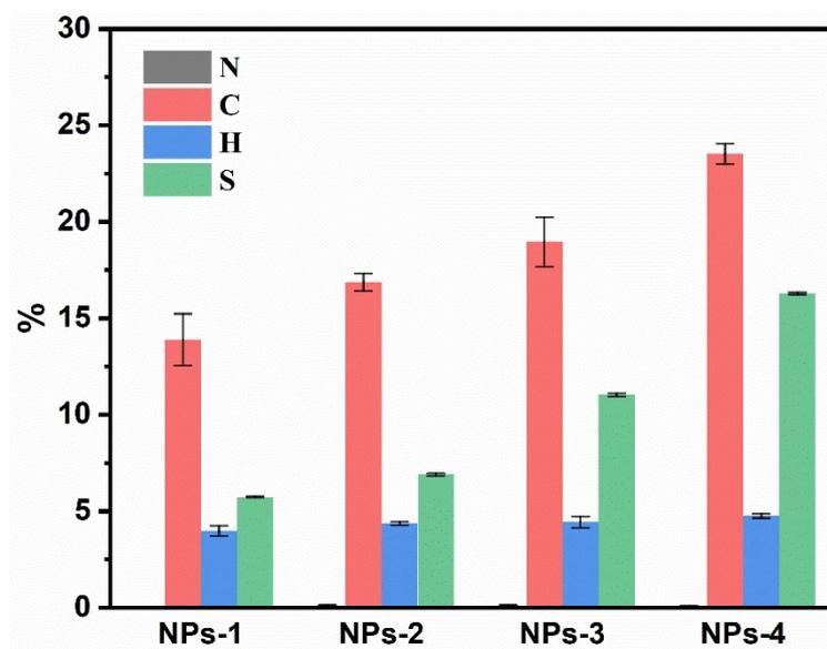
**Fig. S4.** Analysis of N, C, H, and S elements in four thioether-bridged organosilica nanoparticles.
