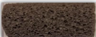
*Figure\_S 1: Pd NPs@glass OCF*
