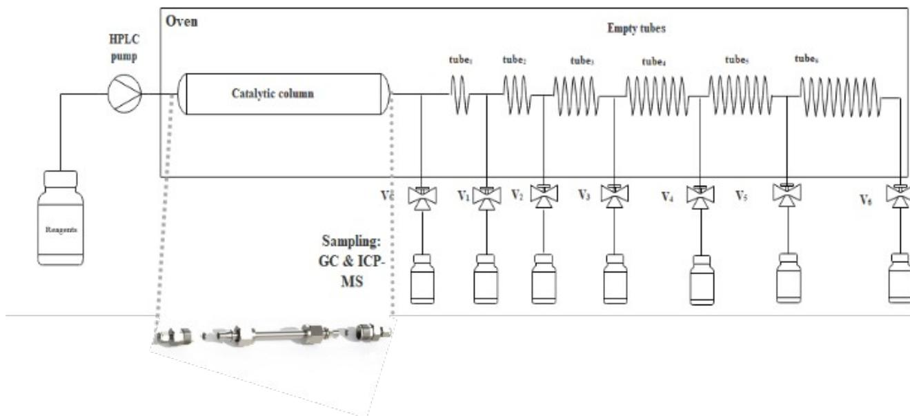
Figure\_S 2: Schematic set-up of the split-flow reactor
