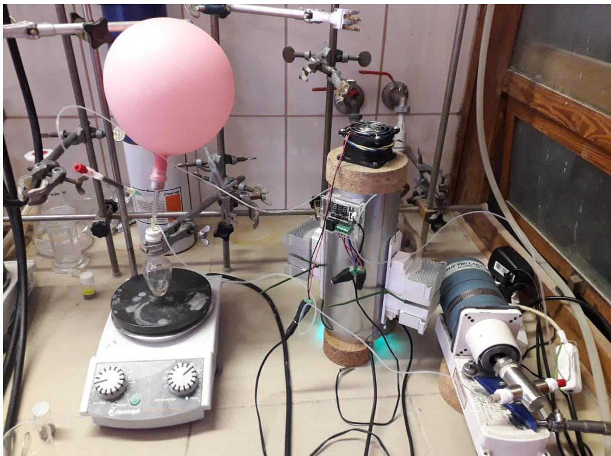
*UV-transparent FEP tubing and column packed with Celite.*
