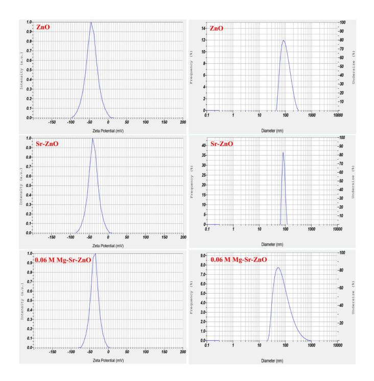
Figure S1. Zeta potential and DLS measurements of the nanocrystals.
