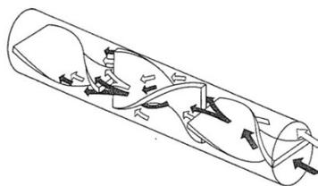
**SI Image 1.** The static mixer coil used in the continuous flow setup for the reactions with KO<sup>t</sup>Bu and NaOMe (left). A schematic of the internal helical structure of the reactor coil which increases reaction mixing (right).
