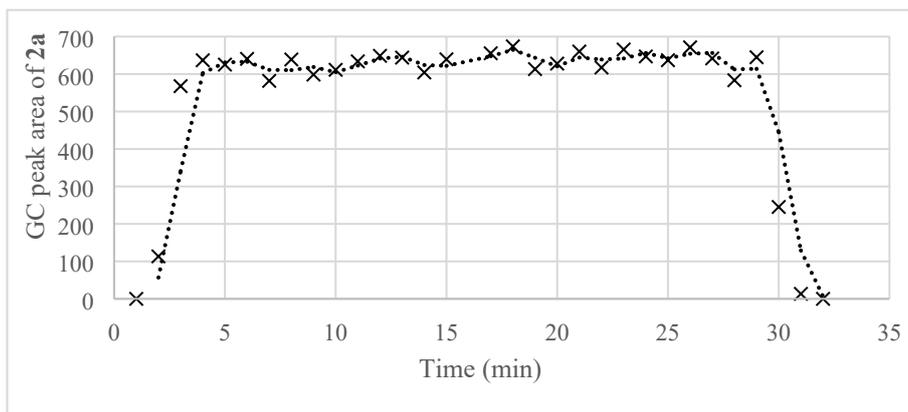
**SI Graph 1.** Steady state plot of the scaled-up reaction (30 mmol). The peak area (plotted on y-axis) was determined *via* GC analysis.
