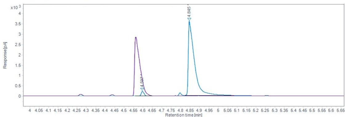
Fig S1: Gas chromatogram (GC) obtained after an 8-hour reaction in the SpinChem reactor using waste-derived Bio1 cells. The purple line represents the chromatogram at t<sub>0</sub> (beginning of the reaction), while the blue line represents the chromatogram at 8 hours. 4.5 minutes: Perillaldehyde retention time; 4.8 minutes: Perillyl-alcohol retention time.
