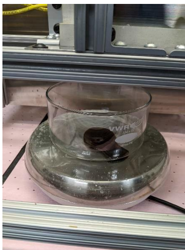
Figure S16. Melt as it exits the plate reactor and is collected on a scale for flow rate measurement and top plate temperature optimization.
