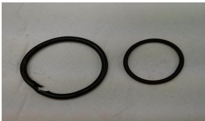
Figure S1: Left: Pump secondary seal exposed overnight to a solution of hydrazine in THF (1 mol/L). Right: Pump secondary seal exposed overnight to THF.
