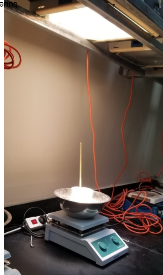
Figure S2: Set up for S. aureus bacterial removal by \text{TiO}_2 photocatalysis
