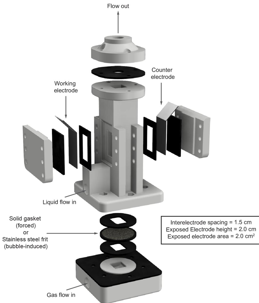
**Fig. S2** Exploded view of flow reactor.
