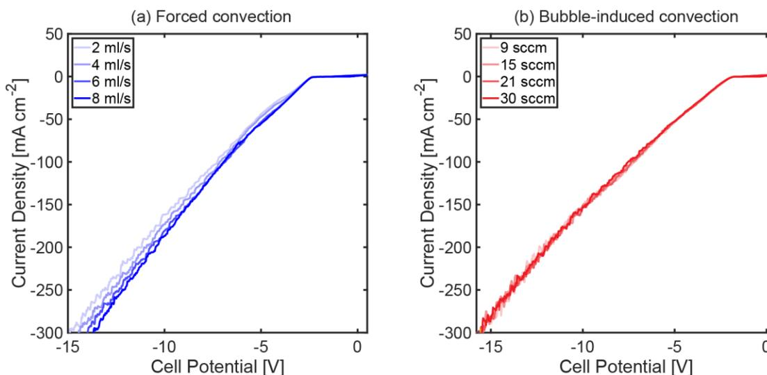
**Fig. S1** Linear sweep voltammetry measurements for (a) forced convection and (b) bubble-induced convection across the range of flow rates used in the experiments.
