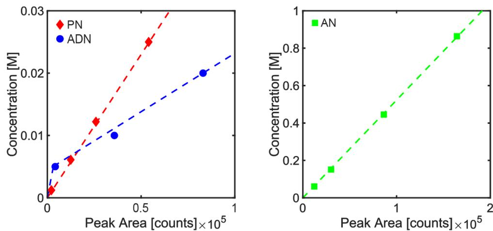
**Fig. S4** GC calibration curves for propionitrile (PN), adiponitrile (ADN), and acrylonitrile (AN) relating GC peak area to concentration. Each point represents an average of 3 samples. The detection limit for ADN is  $\sim 0.004$  M, so the calibration curve has a line to 0 M below 0.005 M to avoid overestimating ADN at low concentrations.
