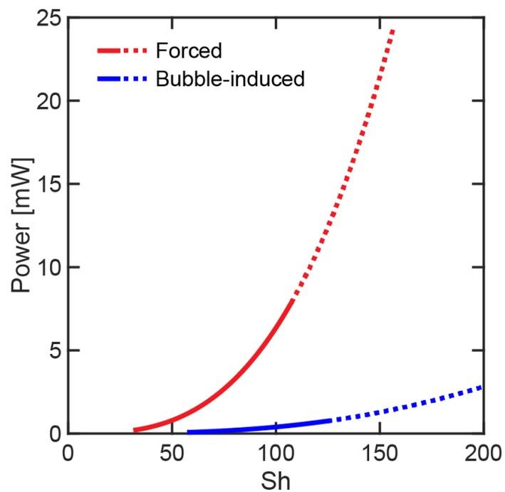
**Fig. S5** Power required to achieve a particular Sherwood number for forced and bubble-induced convection. Solid lines indicate the range of Sherwood numbers attainable for each convection method with the flow rates used in this study, and dashed lines indicate higher Sherwood numbers than those used in this study.
