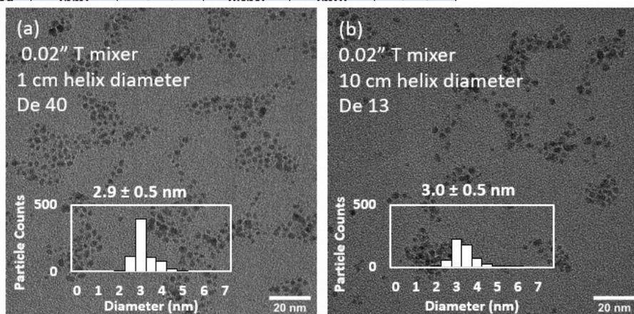
**Figure S.6 Effect of reactor helix diameter on the size and distribution of continuously synthesised Ru NPs. Representative TEM images. Experiments 1 and 6, Table 3.**
