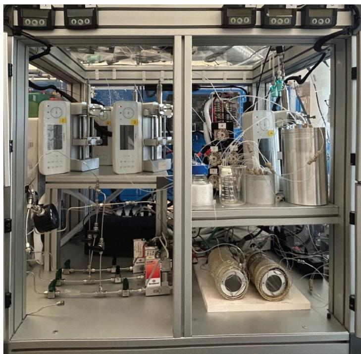
**Figure S2.** A picture of the flow chemistry platform utilized to generate the initial experimental training data. The setup includes a liquid delivery module, a reactive gas manifold, a precursor refilling module, two heated coil flow reactors, and an on-line sampling module (GC-FID).
