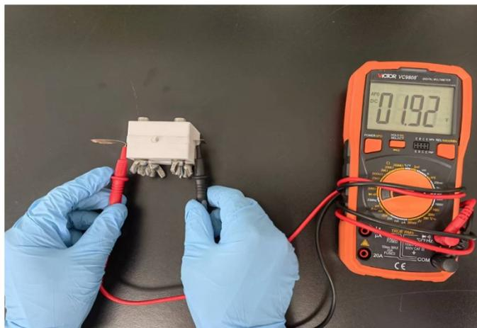
**Figure S30.** Photograph of commercial Pt/C based Al-air battery, with an open circuit potential voltage of 1.92 V.
