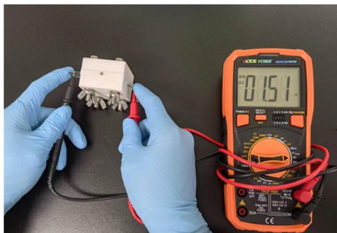
**Figure S31.** Photograph of commercial Pt/C based Zn-air battery, with an open circuit potential voltage of 1.51 V.
