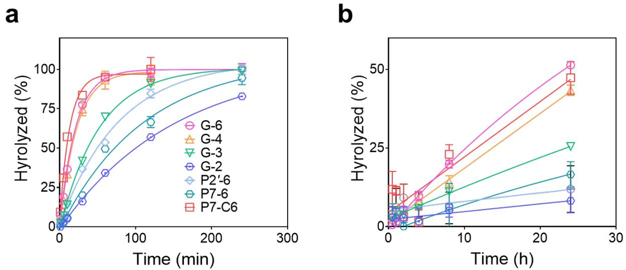
**Figure S35.** Hydrolysis kinetics of Gem and PTX precursors at (a) pH 5.0 and (b) 7.4 ( $n = 4$ ).
