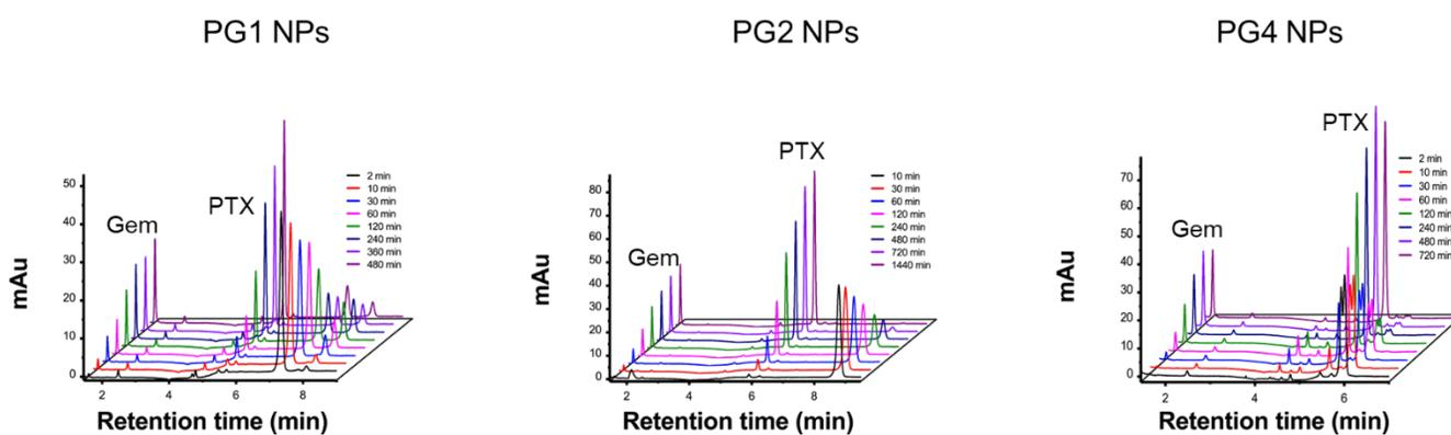
**Figure S37.** The HPLC chromatograms of PG NPs at pH 5.0 over 480 min. Mobile phase was ACN/H<sub>2</sub>O (70/30, v/v); HPLC was run at a flow rate of 1 mL/min. Retention time:  $R_t$  of Gem = 1.6 min;  $R_t$  of PTX = 5.5 min.  $R_t$  of PG1, PG2 and PG4 was 7.2 min, 8.3 min, and 6.9 min.
