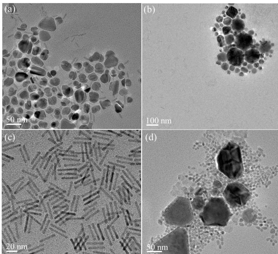
**Figure S5.** Control experiments: (a) TEM image of the products obtained when OLA is used as a reducing reagent without TBAB during reaction. Cu nanocrystals are generated separately from the NRs (homogenous nucleation) (b-d) TEM images of the products obtained by replacing CuOAc with CuBr, CuI or CuCl, respectively.
