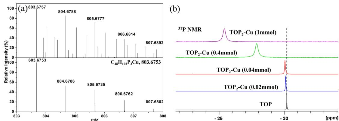
**Figure S8.** (a) Experimental (upper) and calculated (bottom) isotopic distribution at 803 m/z in MS (calculated formula  $C_{48}H_{102}P_2Cu$ ). (b)  $^{31}P$   $\{^1H\}$  NMR spectra of TOP and TOP<sub>2</sub>-Cu complexes synthesized by adding different amount of Cu precursor.
