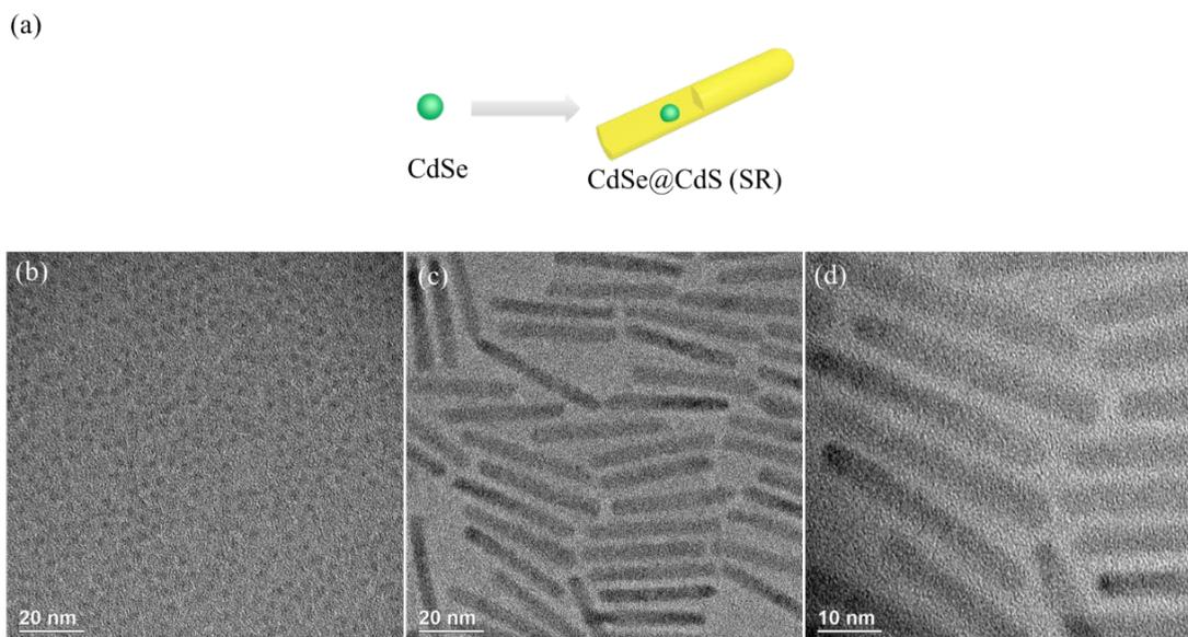
**Figure S1.** (a) illustration of the synthesis of SR. (b) TEM image of primary CdSe seeds with a diameter of about 2.3 nm. (c, d) TEM images of SR under different magnifications.
