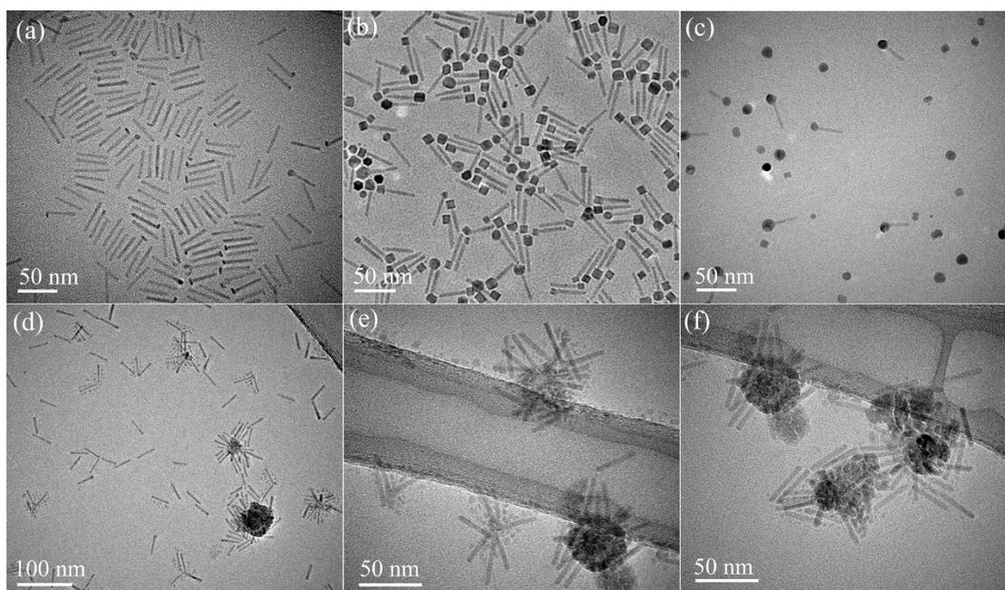
**Figure S3.** TEM images of SR-e-Cu (a), SR-s-Cu (b), SR-c-Cu (c) and SR-Cu multipedes (d-f) taken after 15 months of synthesis.
