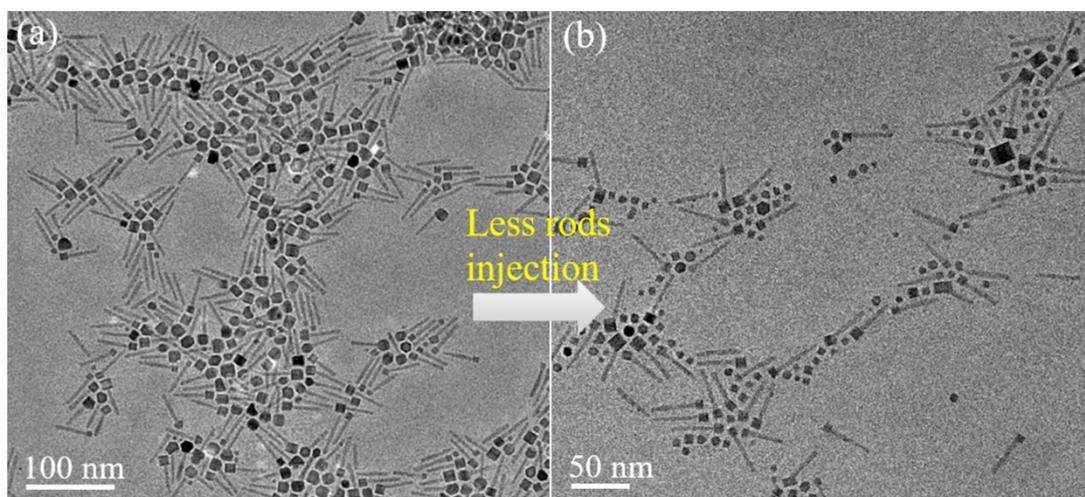
**Figure S2.** (a, b) TEM images of SR-c-Cu heterojunctions synthesized by adding different amount of SR.
