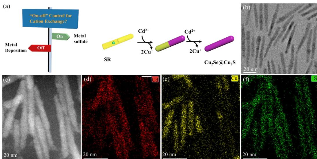
**Figure S7.** (a) illustration of the cation exchange pathway. (b) TEM image of the products obtained by cation exchange (without TOP). (c-f) the HAADF image and its STEM-EDX mapping of the resulting products.
