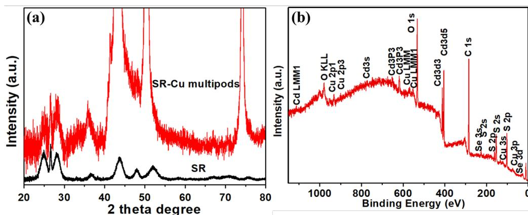
**Figure S4.** (a) XRD patterns of SR-Cu multipods zoomed in on Y axis. (b) XPS survey of the sample.
