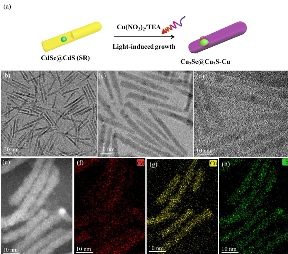
**Figure S6.** (a) Illustration of the photodeposition pathway. (b-d) TEM images of the products by photodeposition (via 455 nm excitation with an LED operating at 200 mW). (e-h) the HAADF image and its STEM-EDX mapping of the resulting products.
