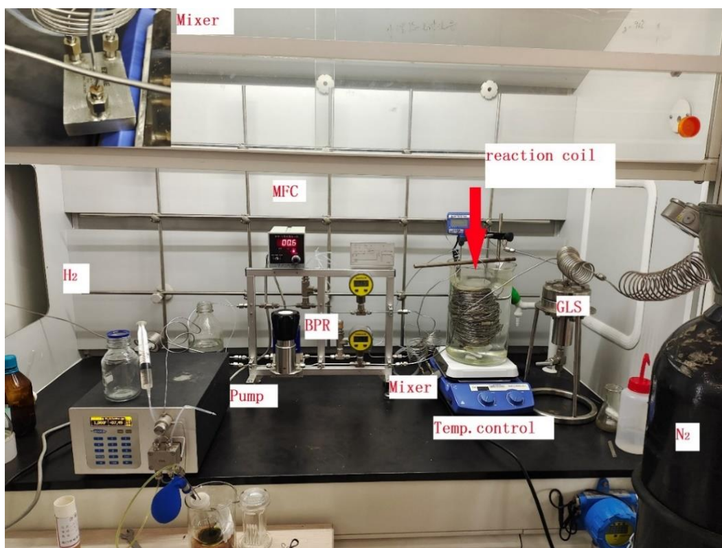
Figure S3. Set-up for asymmetric hydrogenation under continuous flow.
