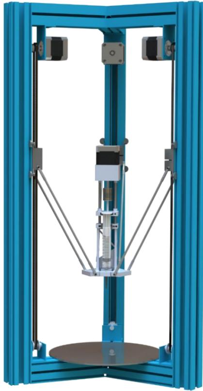
**Fig. S13.** Sol-gel 3D-printer. A laboratory designed and built 3D printer with an advanced extrusion nozzle for precise printing of colloidal sol-gel materials.
