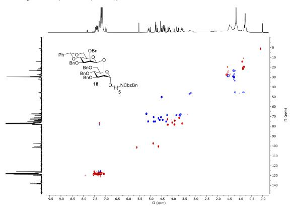
$^1\text{H-}^{13}\text{C}$  Coupled HSQC NMR (400 MHz, CDCl<sub>3</sub>)
