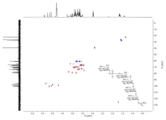
$^{1}\text{H-}^{13}\text{C}$  Coupled HSQC NMR (700 MHz, D<sub>2</sub>O)
