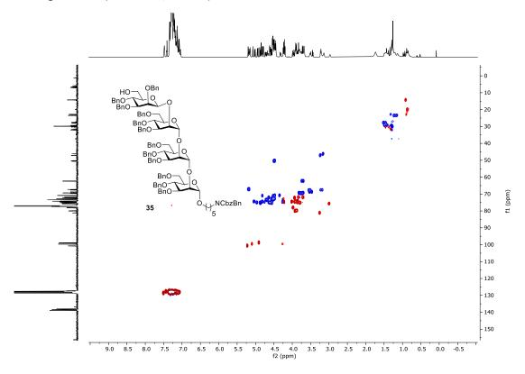
$^1\text{H-}^{13}\text{C}$  Coupled HSQC NMR (700 MHz, CDCl<sub>3</sub>)
