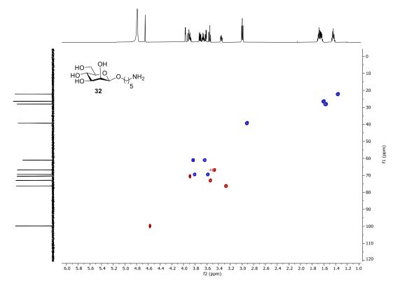
$^{1}\text{H-}^{13}\text{C}$  Coupled HSQC NMR (600 MHz, CDCl<sub>3</sub>)
