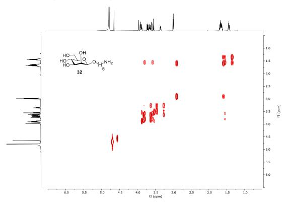
$^{1}\text{H-}^{13}\text{C}$  HSQC NMR (600 MHz, CDCl<sub>3</sub>)
