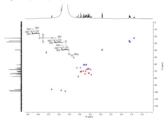
$^{1}\text{H-}^{13}\text{C}$  Coupled HSQC NMR (600 MHz,  $D_{2}\text{O}$ )
