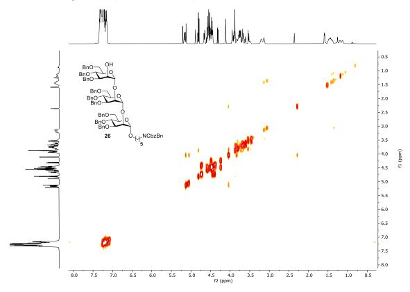
$^{1}\text{H-}^{13}\text{C}$  HSQC NMR (400 MHz, CDCl<sub>3</sub>)
