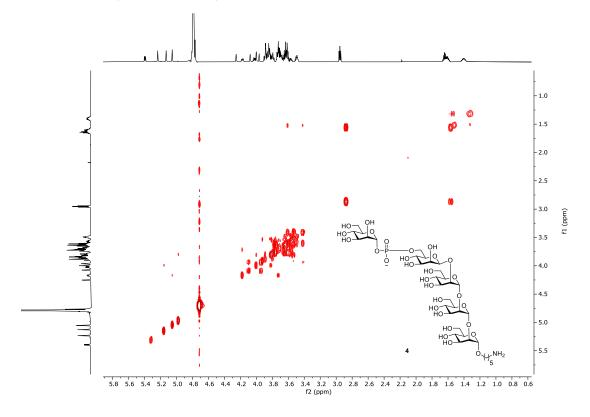
$^{1}\text{H-}^{13}\text{C}$  HSQC NMR (700 MHz, D<sub>2</sub>O)
