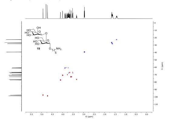
$^{1}\text{H-}^{13}\text{C}$  Coupled HSQC NMR (700 MHz,  $D_{2}\text{O}$ )
