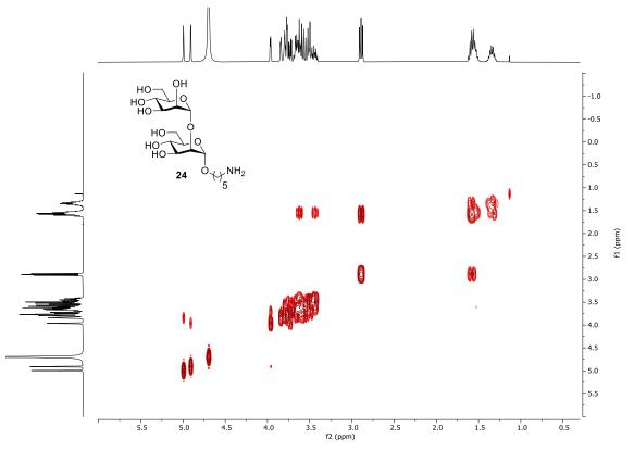
$^{1}\text{H-}^{13}\text{C}$  HSQC NMR (600 MHz,  $D_{2}\text{O}$ )
