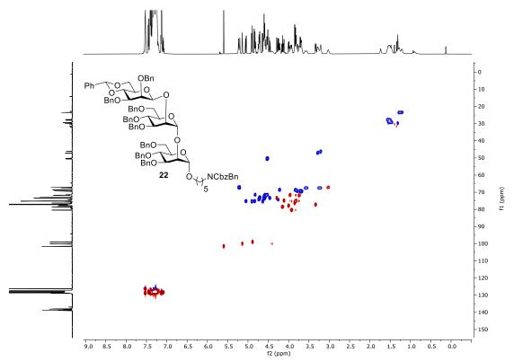
$^{1}\text{H-}^{13}\text{C}$  HSQC NMR (600 MHz, CDCl<sub>3</sub>)
