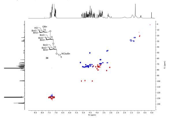
$^1\text{H-}^{13}\text{C}$  Coupled HSQC NMR (400 MHz, CDCl<sub>3</sub>)
