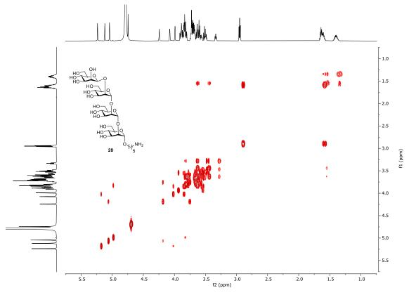
$^{1}\text{H-}^{13}\text{C}$  HSQC NMR (700 MHz, D<sub>2</sub>O)
