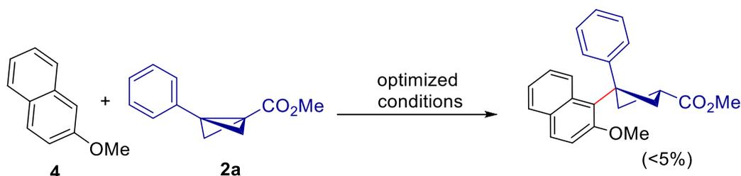
To an oven-dried screw-capped test tube equipped with a magnetic stir bar was added the Bi(OTf)<sub>3</sub> (0.013 g, 0.02 mmol) inside the glove box. After that, 2-methoxynaphthalene **4** (0.032 g, 0.2 mmol) and 1.0 mL CH<sub>2</sub>Cl<sub>2</sub> were added outside the glove box under nitrogen atmosphere. Then the mixture was stirred for 5 minutes at 25 °C. After 5 minutes, methyl 3-
