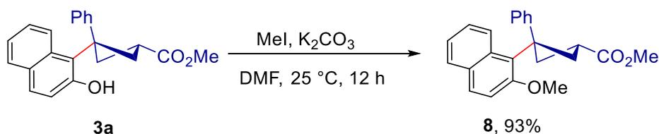
Compound **8** was synthesized following the modified literature procedure.<sup>9</sup> To a solution of **3a** (0.066 g, 0.2 mmol) in 2.0 mL DMF was added K<sub>2</sub>CO<sub>3</sub> (0.041 g, 0.3 mmol) and methyl iodide (0.042 g, 0.3 mmol) then the mixture was stirred at 25 °C for 12 h. Then the solvent was evaporated, and the residue was purified by column chromatography to give methyl-3-(2-methoxynaphthalen-1-yl)-3-phenylcyclobutane-1-carboxylate **8** as a white solid (0.064 g, 93% yield).
