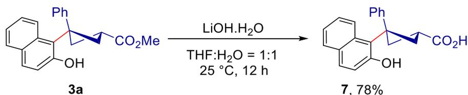
Following the general procedure,<sup>8</sup> methyl-3-(2-hydroxynaphthalen-1-yl)-3-phenylcyclobutane-1-carboxylate **3a** (0.066 g, 0.2 mmol) and lithium hydroxide monohydrate (0.017 g, 0.4 mmol) were dissolved in THF:H<sub>2</sub>O (1+1 mL) at 25 °C and stirred for 12 h. The
