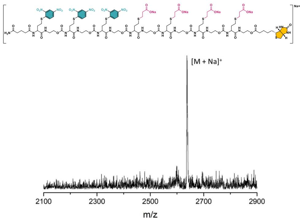
**Figure S3.** MALDI-ToF spectrum of **M3**.  $[M+Na]^+_{\text{calc}} = 2638.55$ ,  $[M+Na]^+_{\text{found}} = 2637.17$
