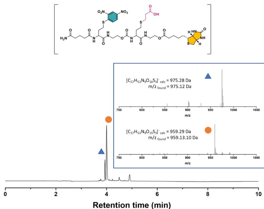
**Figure S2.** LC-MS spectra of **M2** ( $\lambda = 214$  nm). Blue triangle: Thioether oxidation of the desired product.
