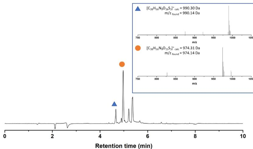
**Figure S1.** LC-MS spectra of **M1** ( $\lambda = 360$  nm). The blue triangle corresponds to the thioether oxidation of the desired product. The two peaks on the right cannot be identified. They do not correspond to truncated structures and are ascribed to a contamination of the LCMS samples.
