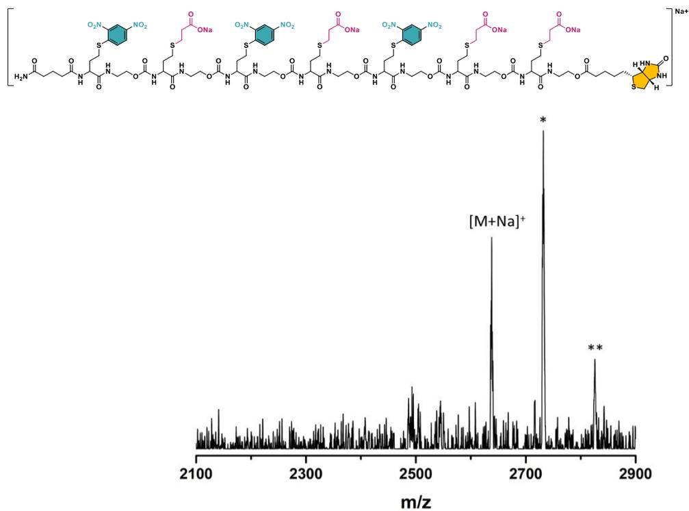
**Figure S4.** MALDI-ToF spectrum of **M4**.  $[M+Na]^+_{\text{calc}} = 2638.55$ ,  $[M+Na]^+_{\text{found}} = 2638.07$ . \* Corresponds to  $[M+TFA+Na]^+$  and \*\* to  $[M+2TFA+Na]^+$ .
