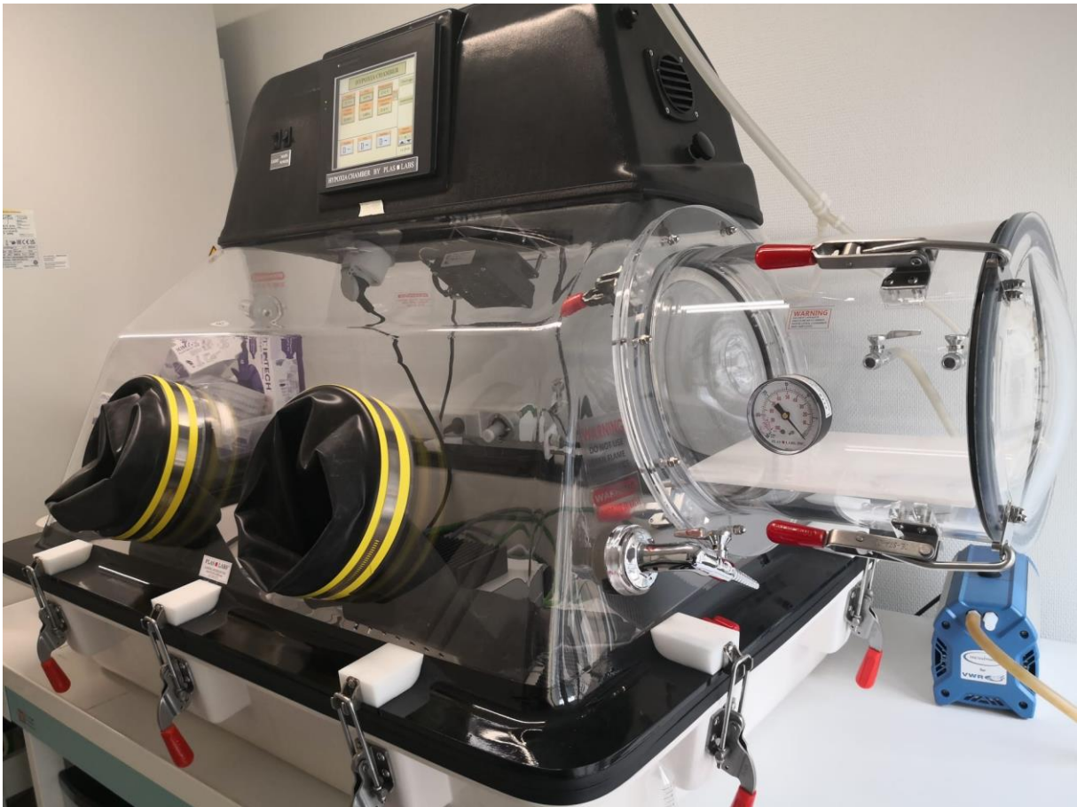
Figure S15. Hypoxia chamber (Plas labs 856-Series hypoxia chamber glove box) containing the irradiation setup.
