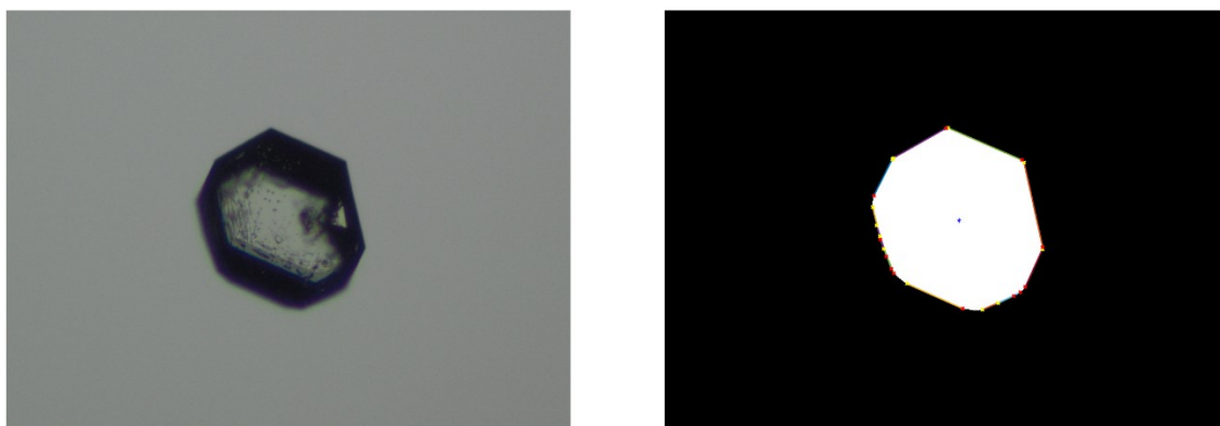
Figure S9. (Left) a grayscale image of a crystal of TFA-IX collected during experiments. (Right) The same image after binarization, edge detection and measurement.
