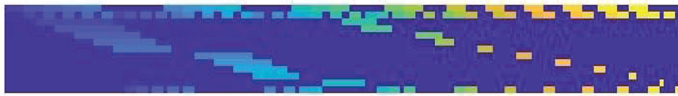
Fig. S6 Visualization of simplified scheduling algorithm in which all operations that occupy the main flowpath were combined. Each unique reaction is represented using a distinct color. Dark blue represents background or unused time. (a) and (b) are both cases in which three reactions being assigned to three parallel reactors, and provide confirmation of the sketch in Figure 4: when the reactions are long compared to the other operations, droplet preparation can be back-to-back (case depicted in (a)); but when reactions are relatively short, as in (b), the algorithm imposes a pause between the preparation of the second and third droplets. (c) shows the algorithm handling a much more complex case, in which twenty reactions are assigned to ten parallel reactors.
