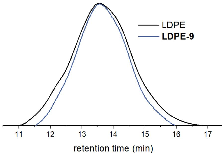
**Figure S30.** The HT-GPC traces. **LDPE** (black),  $M_n = 30423\text{ g/mol}$ ,  $M_w = 177700\text{ g/mol}$ ,  $D = 5.84$ ; **LDPE-9** (blue),  $M_n = 40501\text{ g/mol}$ ,  $M_w = 138482\text{ g/mol}$ ,  $D = 3.42$ .
