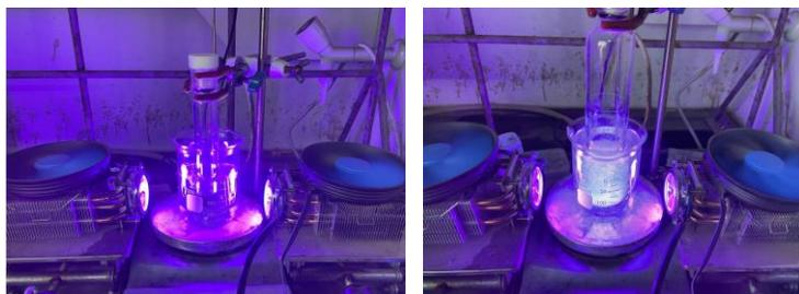
**Figure S2.** The setting-up reactions. Left is for 2-10 mmol scale; right is for > 100 mmol scale.
