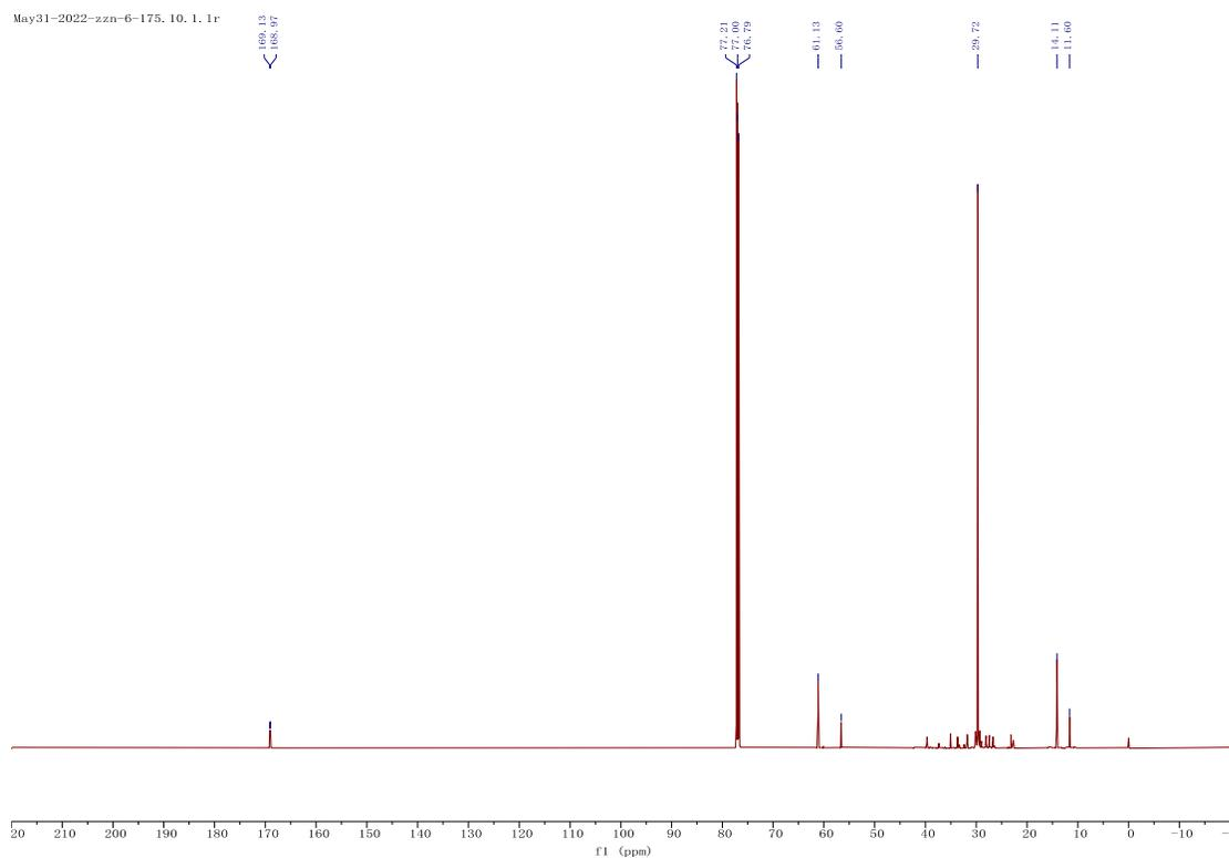
**Figure S38.**  $^{13}\text{C}$  NMR (151 MHz,  $\text{CDCl}_3$ ) of LDPE-11
