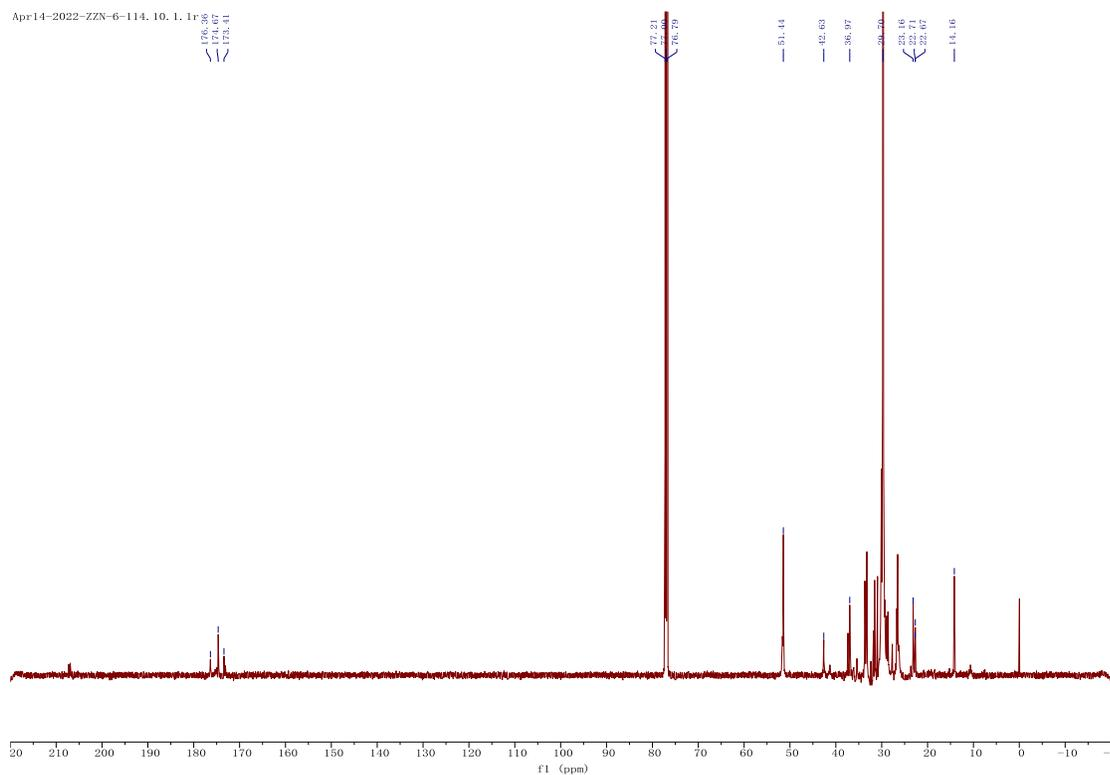
**Figure S5.**  $^{13}\text{C}$  NMR (151 MHz,  $\text{CDCl}_3$ ) of LDPE-5
