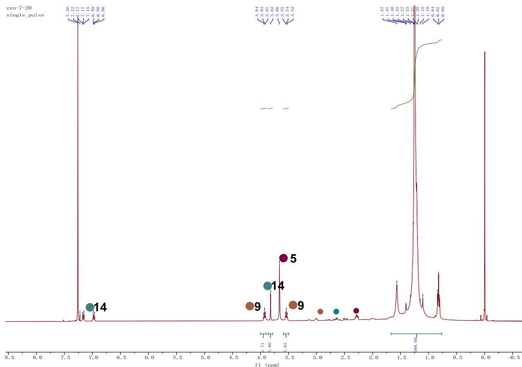
**Figure S87.**  $^1\text{H}$  NMR (400 MHz,  $\text{CDCl}_3$ ) of LLDPE-5-14-9
