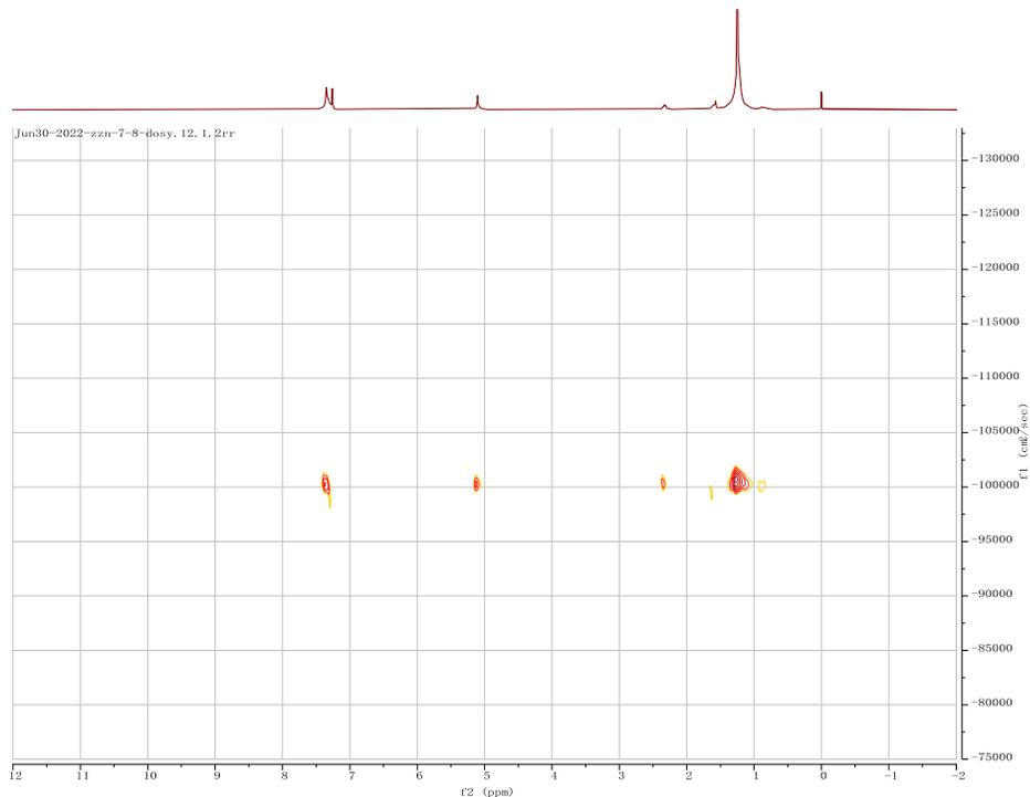
**Figure S19.** Diffusion ordered NMR spectroscopy (DOSY) of **LDPE-6** presented that the all protons of **LDPE-6** had the same diffusion coefficient, indicating the small molecule is covalently linked onto LDPE.
