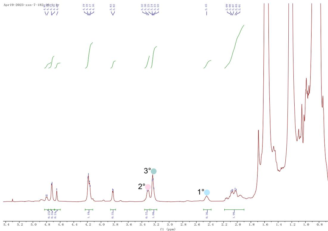
**Figure S56.**  $^1\text{H}$  NMR (400 MHz,  $\text{CDCl}_3$ ) of benzalmalononitrile alkylation products with PP.
