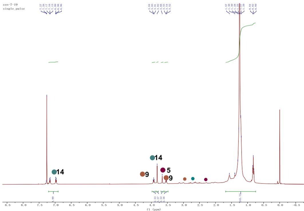
**Figure S80.**  $^1\text{H}$  NMR (400 MHz,  $\text{CDCl}_3$ ) of LLDPE-5-14-9
