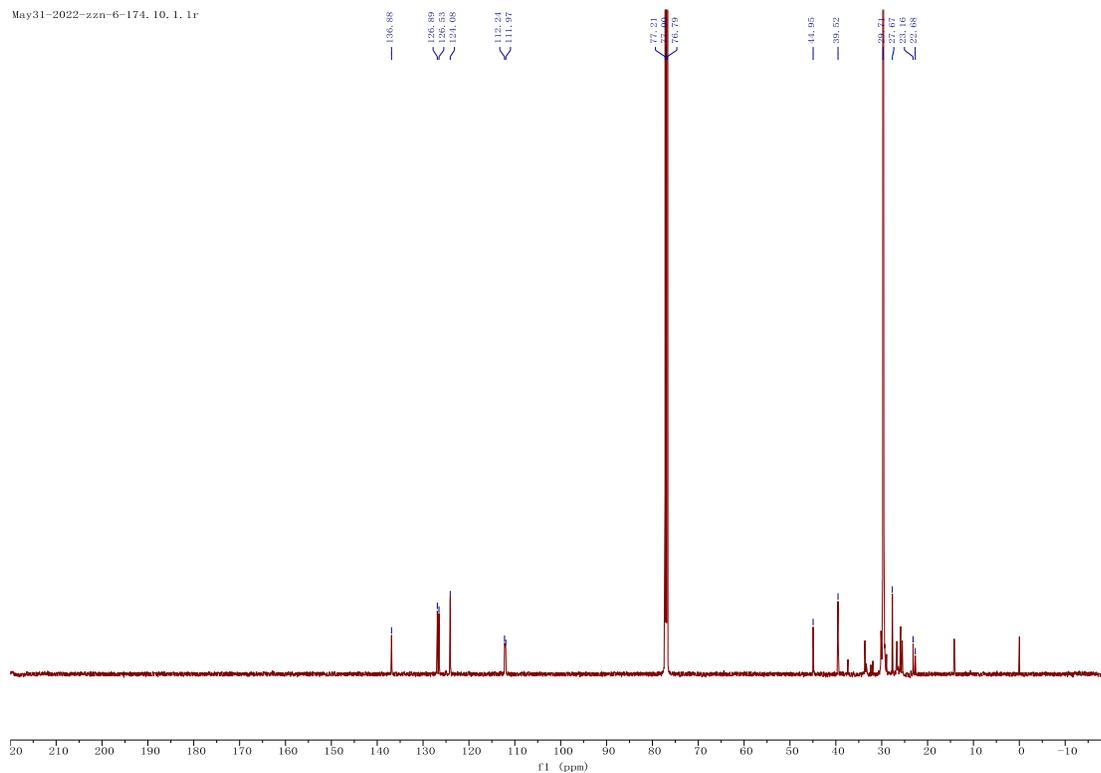
**Figure S41.**  $^{13}\text{C}$  NMR (151 MHz,  $\text{CDCl}_3$ ) of LDPE-12
