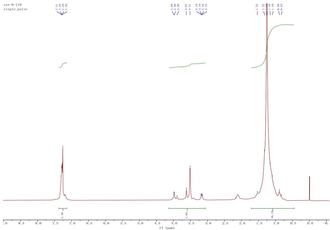
**Figure S44.**  $^1\text{H}$  NMR (400 MHz,  $\text{CDCl}_3$ ) of LDPE-13
