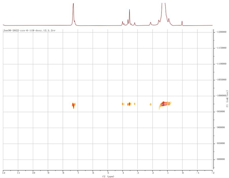
**Figure S47.** Diffusion ordered NMR spectroscopy (DOSY) of **LDPE-13** presented that the all protons of **LDPE-13** had the same diffusion coefficient, indicating the small molecule is covalently linked onto LDPE.
