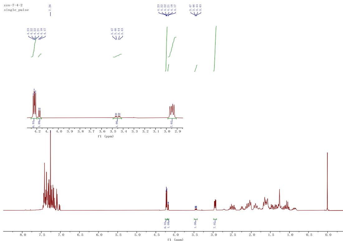
**Figure S62.**  $^1\text{H}$  NMR (400 MHz,  $\text{CDCl}_3$ ) of benzalmalononitrile alkylation products with cyclohexylbenzene (more polar mixture)
