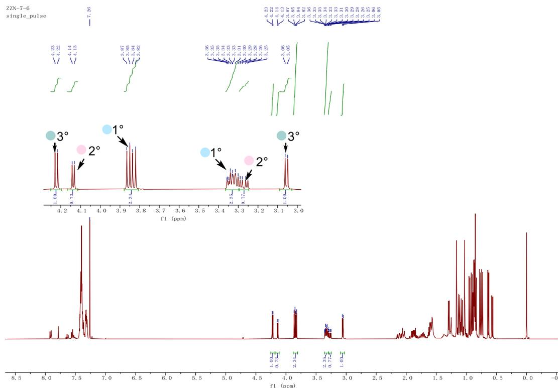
**Figure S55.**  $^1\text{H}$  NMR (400 MHz,  $\text{CDCl}_3$ ) of benzalmalononitrile alkylation products with 2,4-dimethylpentane
