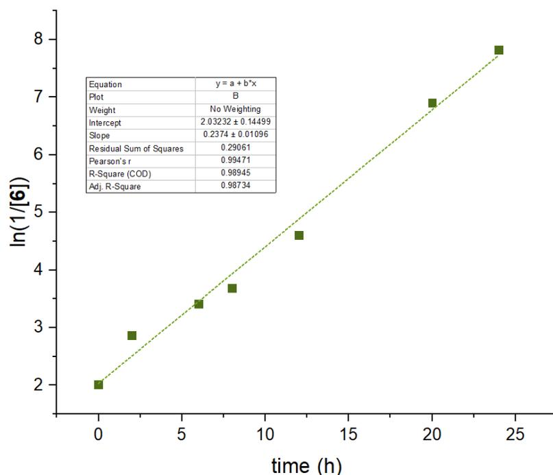
**Figure S10.** A linear relationship was observed for  $\ln(1/[6])$  vs reaction time, indicating a first order dependence of the reaction rate with alkene **6**.
