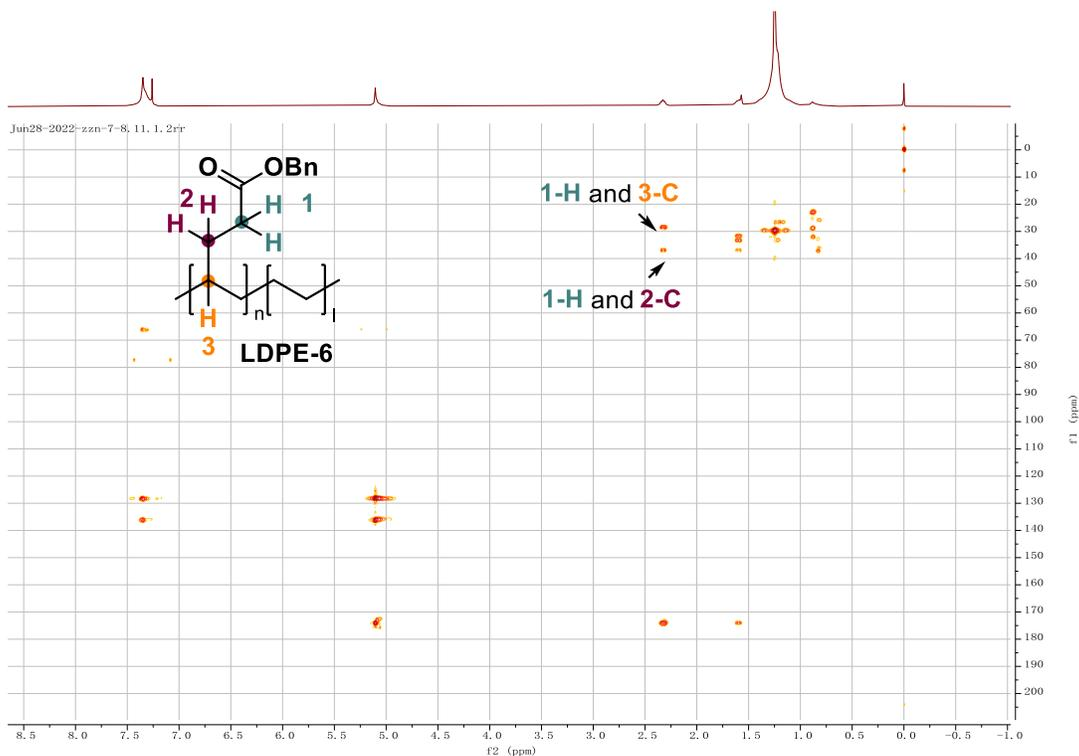
**Figure S18.** Heteronuclear multiple bond correlation (HMBC) spectroscopy of **LDPE-6**.
