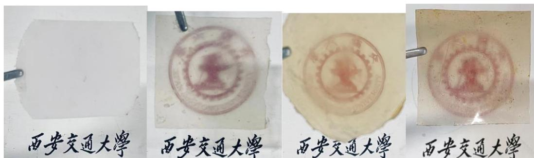
**Figure S103.** Images of LLDPE, *ion*-LLDPE-16, *ion*-LLDPE-9-0.7 mol%, and *ion*-LLDPE-9-2.4 mol% films. Comparing with LLDPE, the clarity of ionized-LLDPE is enhanced.
