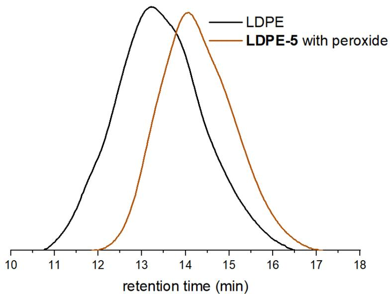
**Figure S9.** The HT-GPC traces of comparable result using BPO as a radical initiator
