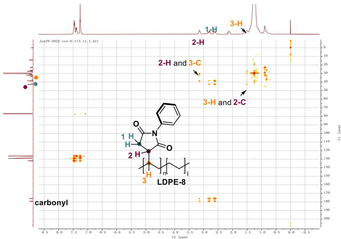
**Figure S28.** Heteronuclear multiple bond correlation (HMBC) spectroscopy of **LDPE-8**
