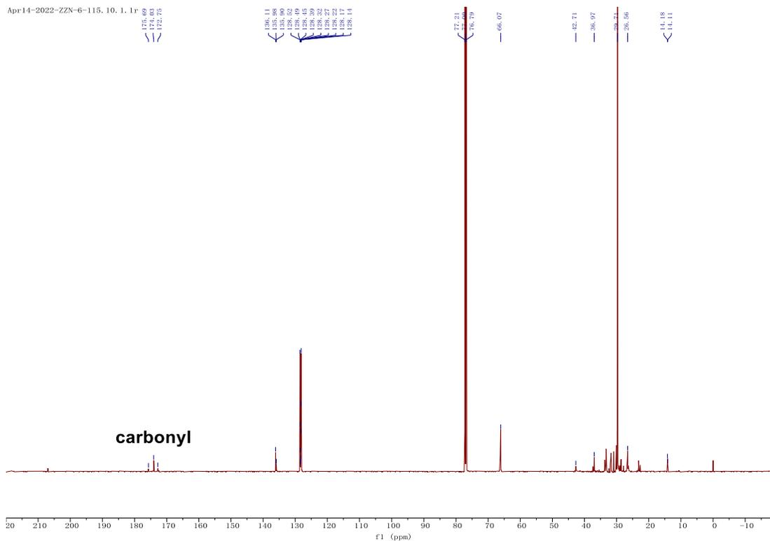
Figure S17.  $^{13}\text{C}$  NMR (151 MHz,  $\text{CDCl}_3$ ) of LDPE-6
