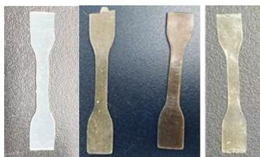
**Figure S104.** Images of LLDPE, *ion*-LLDPE-9-0.7 mol%, *ion*-LLDPE-9-2.4 mol%, and *ion*-LLDPE-16 dog-bones for tensile test.
