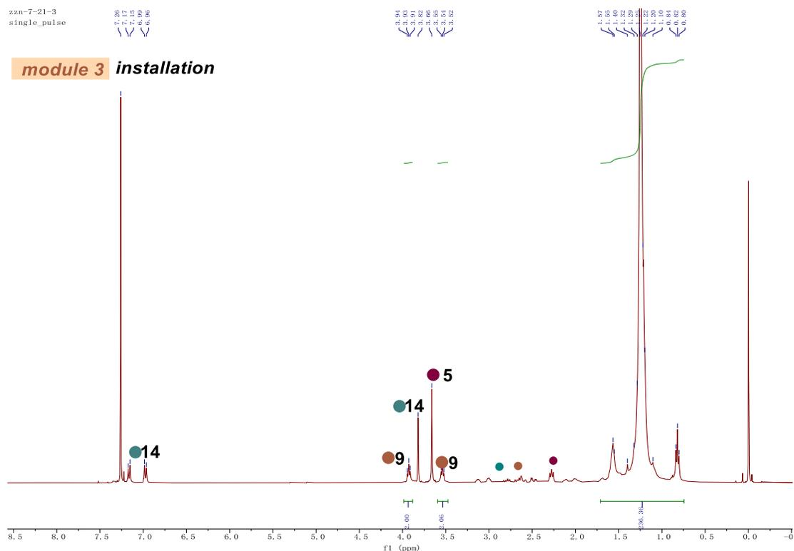
**Figure S78.**  $^1\text{H}$  NMR (400 MHz,  $\text{CDCl}_3$ ) of **LLDPE-5-14-9**
