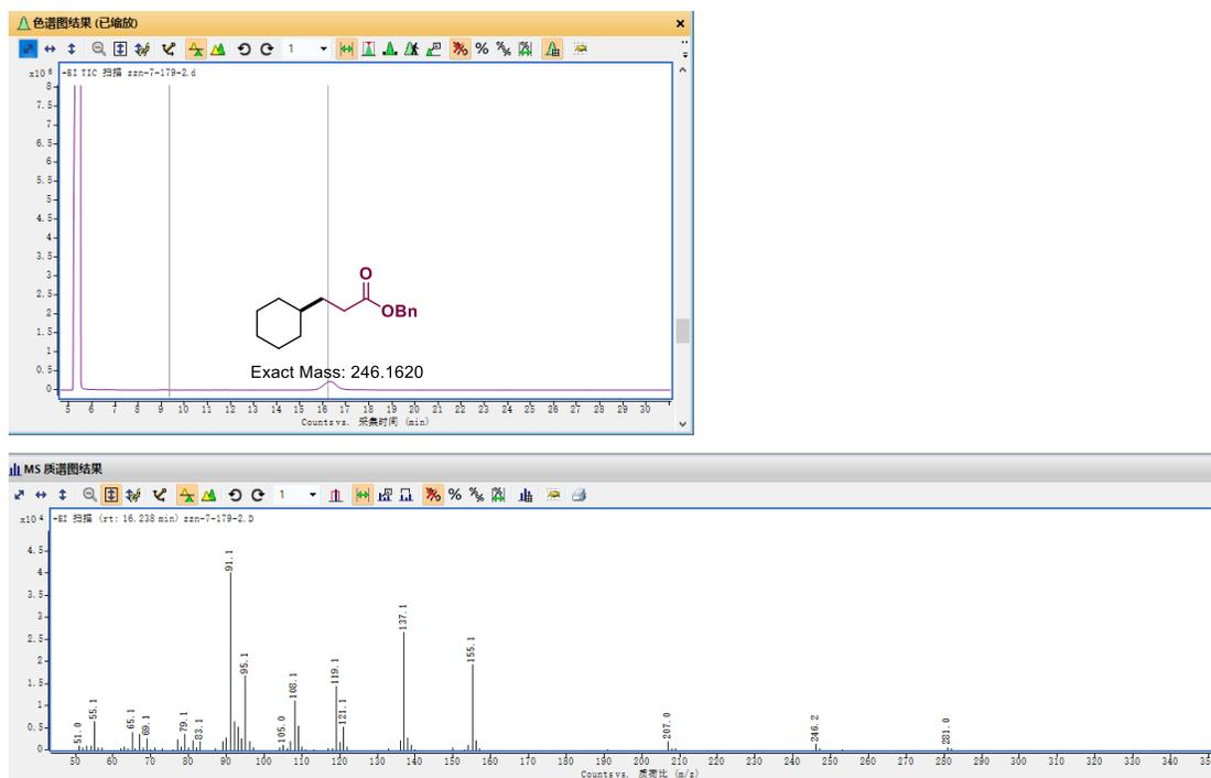
Figure S13. The detection of cross-coupling product by GC-MS.
