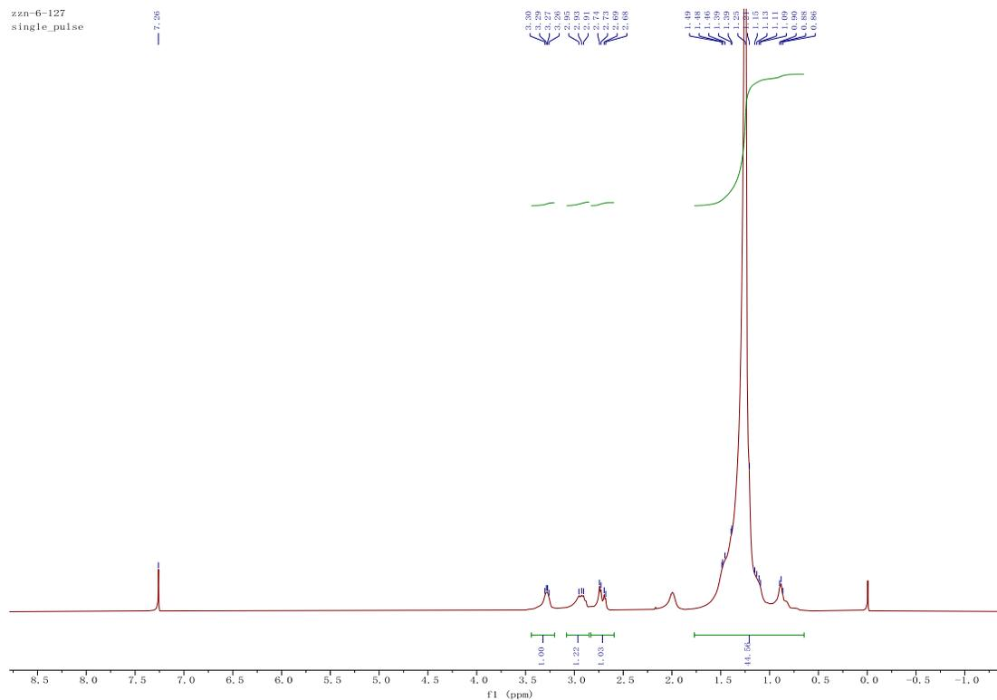
**Figure S34.**  $^1\text{H}$  NMR (400 MHz,  $\text{CDCl}_3$ ) of LDPE-10
