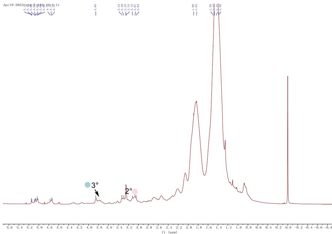
**Figure S63.**  $^1\text{H}$  NMR (400 MHz,  $\text{CDCl}_3$ ) of benzalmalononitrile alkylation products with PS.
