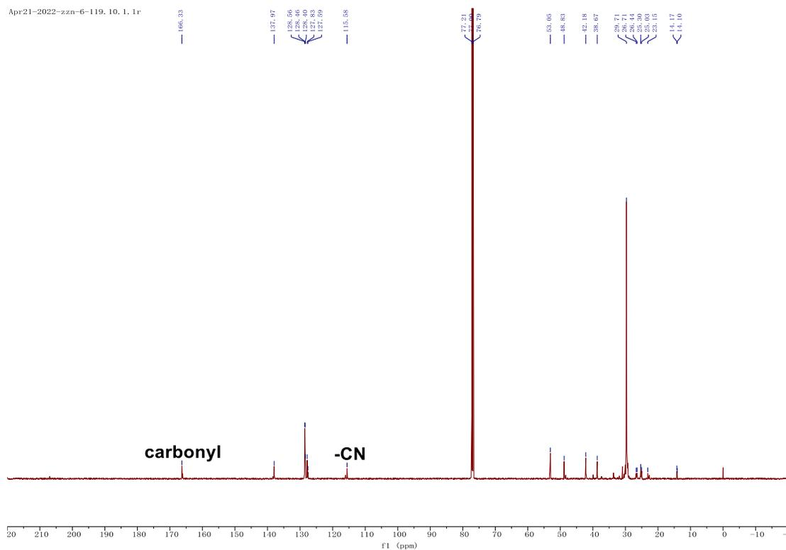
**Figure S45.**  $^{13}\text{C}$  NMR (151 MHz,  $\text{CDCl}_3$ ) of LDPE-13
