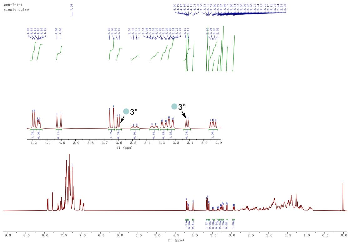
**Figure S61.** <sup>1</sup>H NMR (400 MHz, CDCl<sub>3</sub>) of benzaldehyde malononitrile alkylation products with cyclohexylbenzene (less polar mixture)
