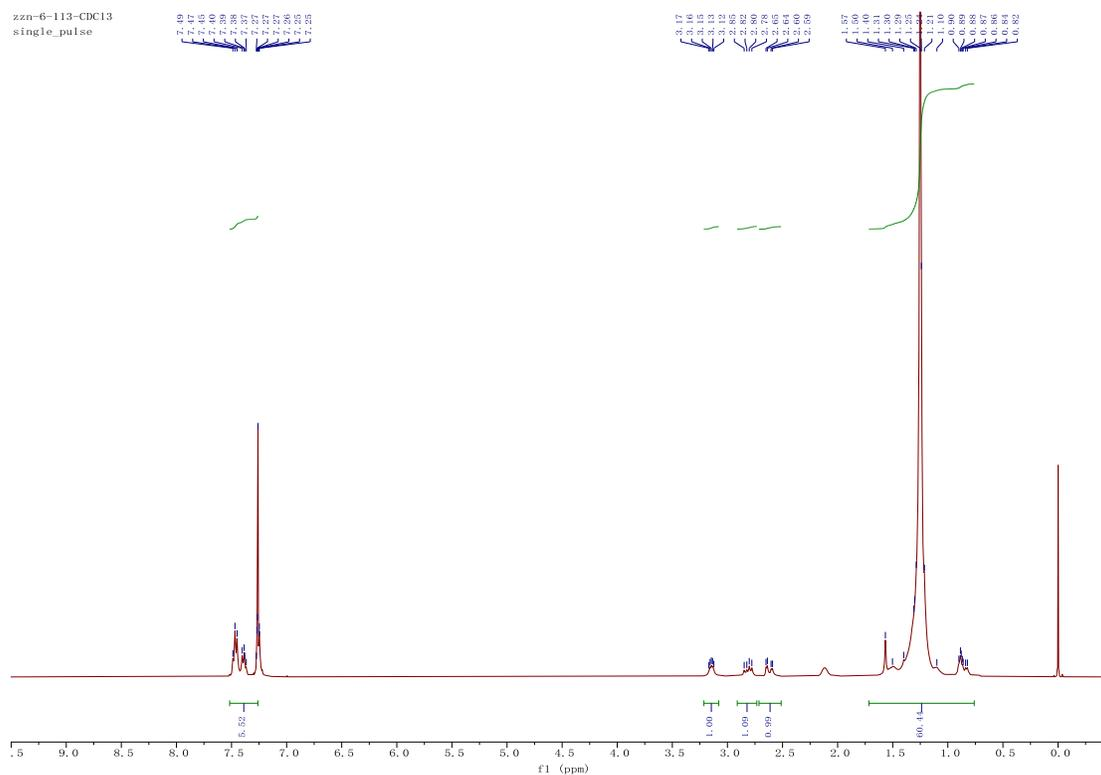
**Figure S26.** <sup>1</sup>H NMR (400 MHz, CDCl<sub>3</sub>) of LDPE-8
