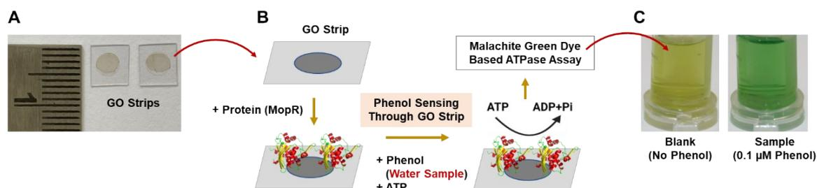
**Figure S3.** (A) GO-D3 coated strips for protein immobilization. (B) Schematic illustration of the MopR immobilization on the GO-D3 strips and ATPase assay. (C) Real-time colour development of the biosensor achieved through malachite green dye-based assay for phenol detection.
