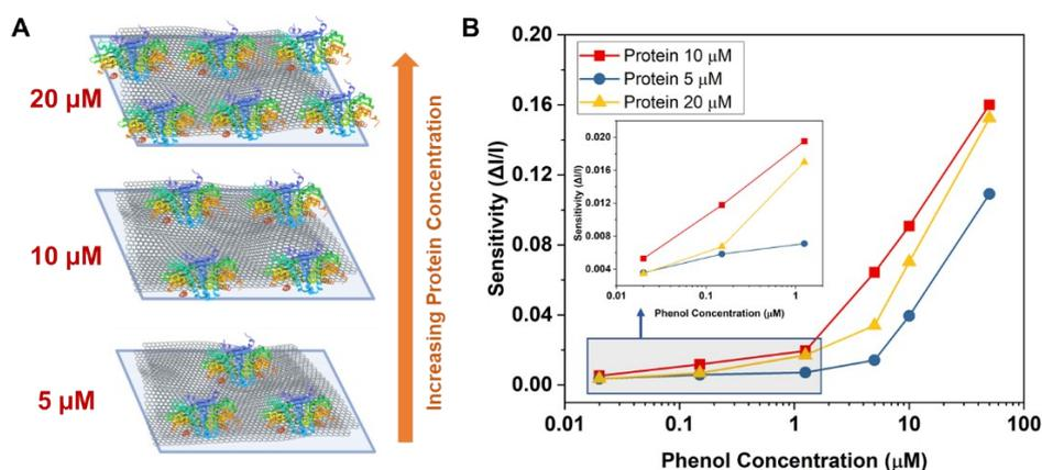
**Figure S11.** Optimization of the biosensing protein (MopR) concentration on the gate electrode. (A) Schematic representation of the different protein concentrations showing increasing crowding. (B) The sensitivity response of the device for different MopR concentration.
