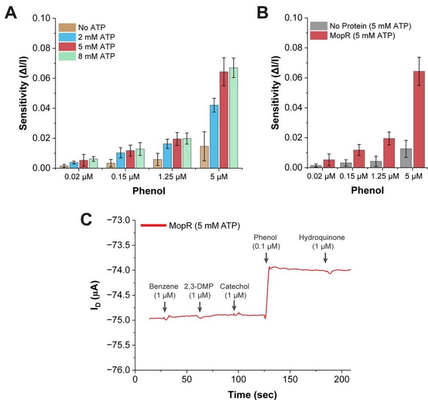
**Figure S9.** (A) Phenol sensitivity of the OECT device at different concentrations of ATP. (B) Sensitivity of the phenol detection response of the ‘no protein’ and ‘protein (MopR) immobilized’ device. (C) Time-channel current ( $I_D$ ) response of the device for different isostructural compounds exhibiting selectivity for phenol.
