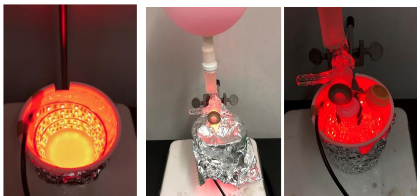
Figure S1. Reaction setup. (a, left) a strip of LEDs is coiled on inner face of plastic cup. (b, center) (c, right) the reaction flask is irradiated by red LEDs.
