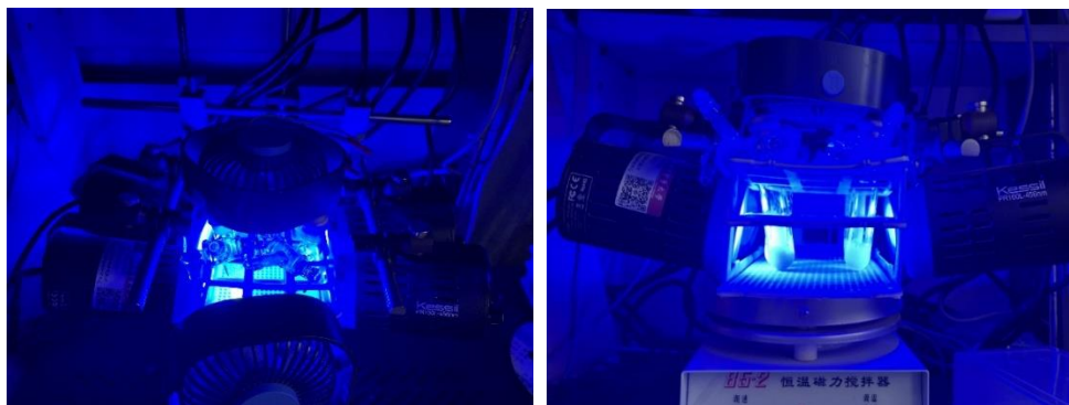
Figure S1: Photochemical reaction setup using 456 nm Kessil Lamps.
