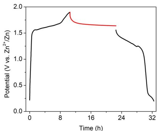
**Figure S2.** Self-discharge performance of the  $\text{Zn}^{2+}$ -trapped  $\text{Mn}_3\text{O}_4$  electrode after being charged in the 20 *m*  $\text{ZnCl}_2$  + 5 *m*  $\text{NH}_4\text{Cl}$  WiSE. The red portion of the curve shows the self-discharge behavior while resting the cell for 12 hours. Cycling was done using a  $\text{Mn}_3\text{O}_4$  free-standing film electrode at 100 mA/g. The Coulombic efficiency after idling the cell was 94.3%.
