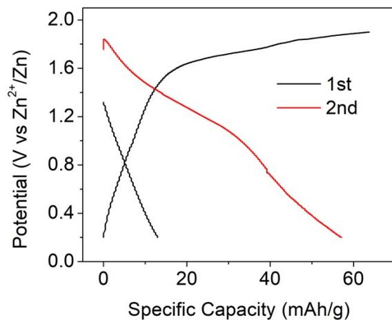
**Figure S4.** GCD profiles of the  $\text{Mn}_3\text{O}_4$  electrode obtained at 50 mA/g using 15 *m* TEACl as the aqueous electrolyte. Activated carbon was used as the counter electrode and Ag/AgCl was used as the reference electrode. Reference potentials were converted to being vs  $\text{Zn}^{2+}/\text{Zn}$  for comparison.
