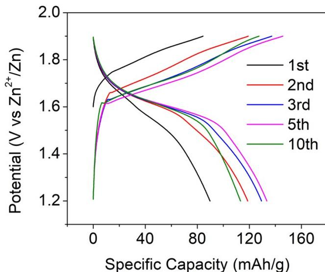
**Figure S3.** GCD profiles of the first, second, third, fifth, and tenth cycles of the  $\text{Mn}_3\text{O}_4$  electrode without initially trapping  $\text{Zn}^{2+}$  ions (charging first and increasing the lower cutoff potential to 1.2 V) at a current rate of 50 mA/g.
