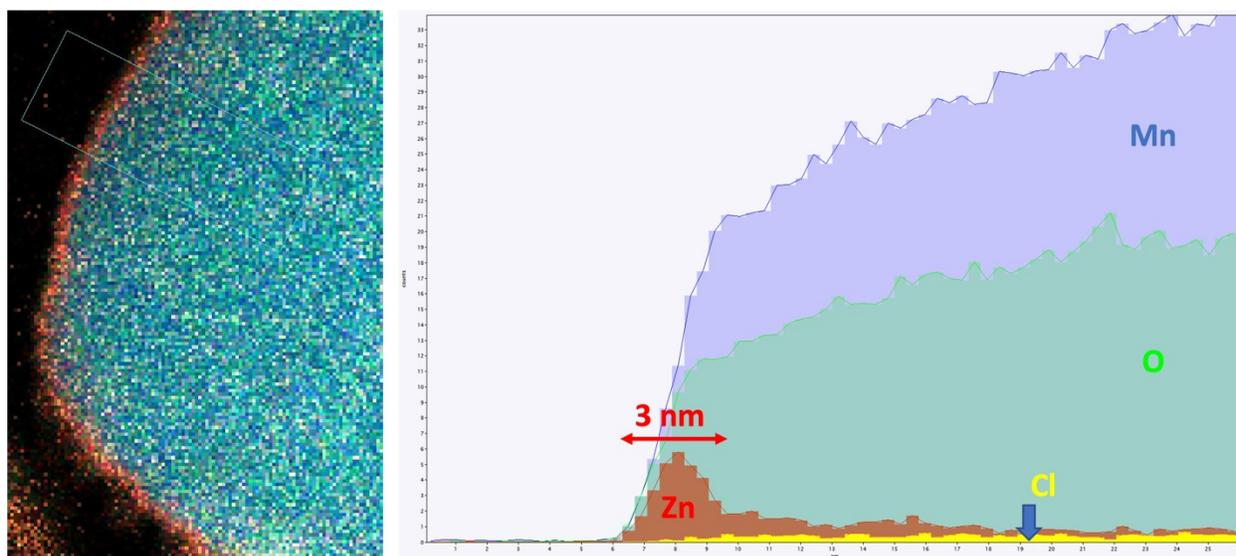
**Figure S7.** EDS line scanning profile of the  $\text{Mn}_3\text{O}_4$  electrode after the first charge. The Mn, O, and Cl contents are distributed fairly uniform throughout the particle, whereas the Zn content is concentrated toward the outer 3 nm of the particle.
