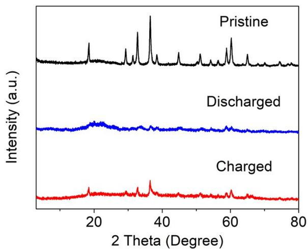
**Figure S6.** XRD patterns of the pristine, discharged, and charged  $\text{Mn}_3\text{O}_4$  electrodes in the WiSE.
