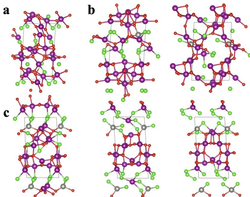
**Figure S10.** Possible optimized structures of Cl intercalation in (a) pristine Mn<sub>3</sub>O<sub>4</sub>, (b) ZnOh, and (c) ZnTd.
