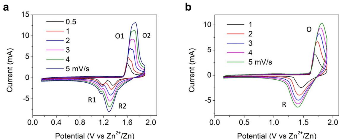
**Figure S5.** CV curves of the  $\text{Mn}_3\text{O}_4$  electrode in (a) 2 M  $\text{ZnSO}_4$  and (b) 20 *m*  $\text{ZnCl}_2$  + 5 *m*  $\text{NH}_4\text{Cl}$  electrolytes at a scan rate of 1 mV/s.
