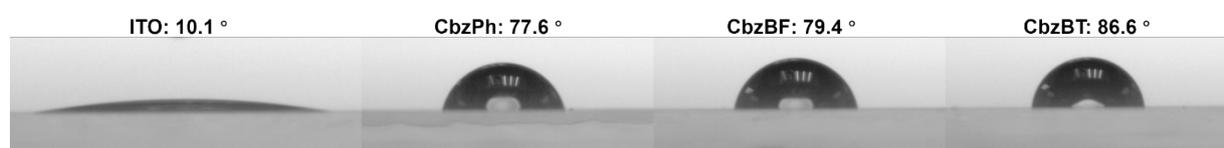
**Figure S13.** Water contact angles of bare ITO, CbzPh-, CbzBF- and CbBT-modified ITO.
