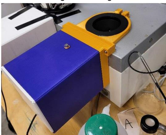
4. Clamp the enclosure to the EasyMax reactor.
