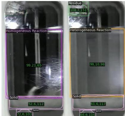
Figure S4. Images from early model development showing “solid” class at the bottom of EasyMax reactor.
