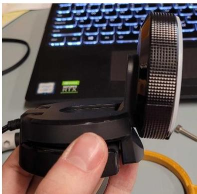
b. Tilt the second joint as far towards the front of the enclosure as it will go. Take the camera stopper and screw it into the top of the enclosure behind the camera. The side with the slant should face the front of the enclosure.
