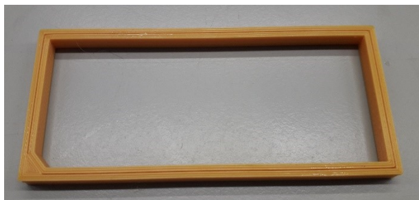
Fig. S 3 3D printed PLA frame with cut off corner to maintain the position of Sample #1 in the sample set.
