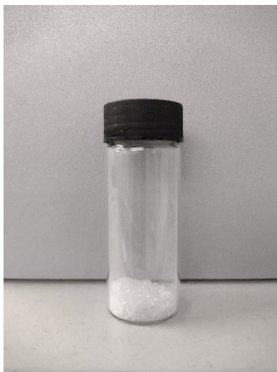
Figure S1.1: Powdered glass prepared from a Fisher Scientific borosilicate glass Pasteur pipette.
