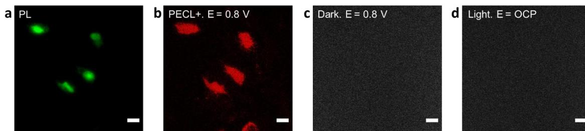
**Figure S3.** Microscopy images of CHO-K1 cells labeled with SA@Ru in a) PL, b) in PECL+ at 0.8 V in ProCell solution on  $n$ -Si/SiO<sub>x</sub>/Ir electrode under infrared light. Control experiment showing the images recorded c) in the dark at 0.8 V and d) under infrared light at open circuit potential (OCP). Scale bar = 20  $\mu\text{m}$ .
