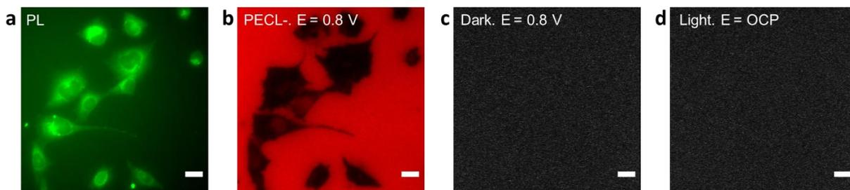
**Figure S7.** Microscopy pictures of CHO-K1 cells labeled with calcein-AM in a) FL, b) PECL- at 0.8 V in PBS containing 30  $\mu\text{M}$   $[\text{Ru}(\text{bpy})_3]^{2+}$  and 0.1 M TPrA on  $n\text{-Si}/\text{SiO}_x/\text{Ir}$  electrode under infrared light. Control experiment showing the images recorded c) in the dark at 0.8 V and d) under infrared light at open circuit potential (OCP). Scale bar = 20  $\mu\text{m}$ .
