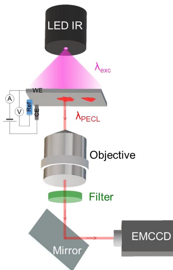
**Figure S1.** Scheme of the PECL set-up on an inverted epi-fluorescence microscope using a near-infrared LED in back-illumination.
