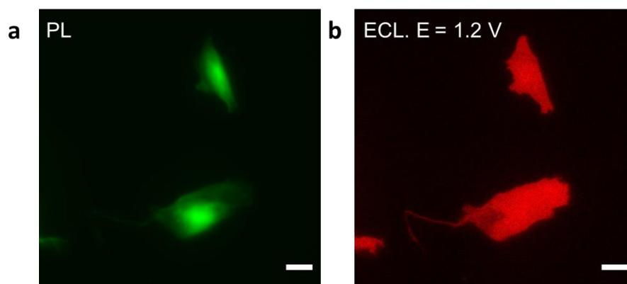
**Figure S2.** Microscopy images of CHO-K1 cells labeled with SA@Ru in a) PL and in b) ECL at  $E = 1.2 \text{ V}$  (vs Ag/AgCl) in ProCell solution on  $p^{++}$ -Si/SiO<sub>x</sub>/Ir electrode. Scale bar: 20  $\mu\text{m}$ . Same region of interest (i.e. same cells) as Figure 4a,b.
