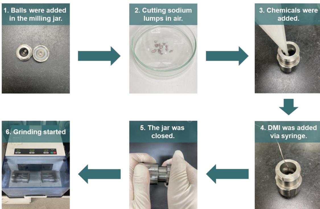
**Figure S3.** Set-up procedure for mechanochemical Birch reduction.
