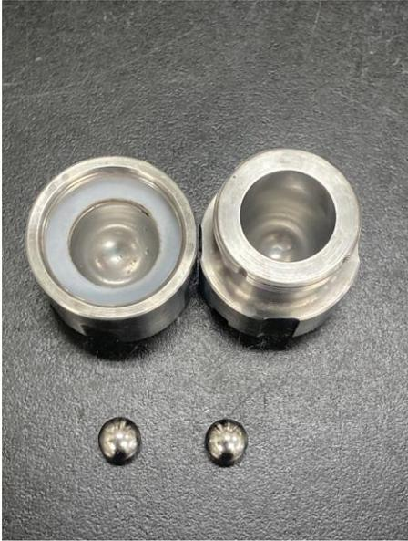
**Figure S2.** Stainless jar (10 mL) and balls (10 mm) used in this study.
