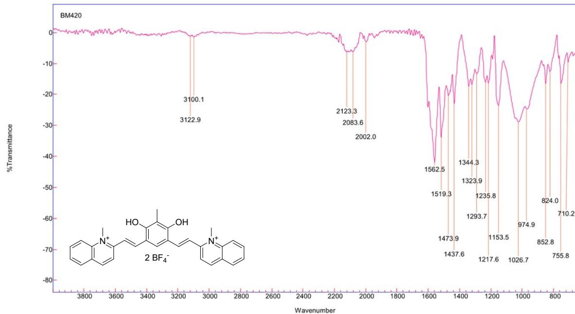
Figure S 65. Infrared spectrum of compound **4•2H<sup>2+</sup>** (neat).
