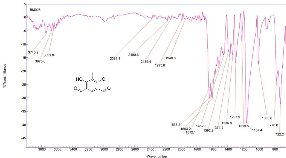
Figure S 54. Infrared spectrum of compound 6 (neat).
