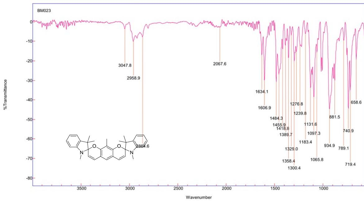
Figure S 60. Infrared spectrum of compound **dsp-1** (neat).
