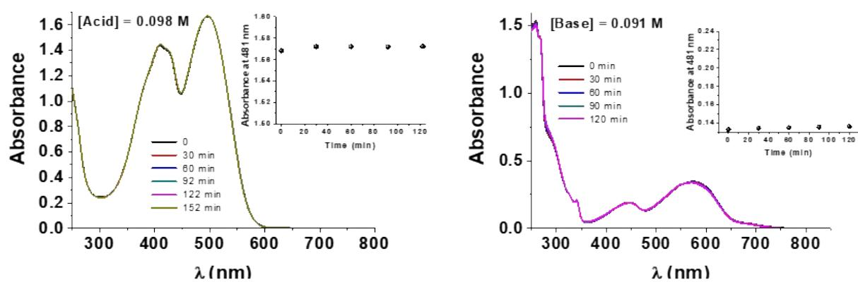
Figure S 81. (A) UV-visible absorption spectra as a function of time measured for  $\mathbf{1}$  in  $\text{CH}_3\text{OH}/\text{H}_2\text{O}$  (80:20 by weight) under acidic (left) and basic (right) conditions for solutions exposed in the dark.  $I = 0.1 \text{ M NBu}_4\text{ClO}_4$ ;  $T = 25.0 \pm 0.1 \text{ }^\circ\text{C}$ ;  $[1] = 2.28 \times 10^{-5} \text{ M}$ .
