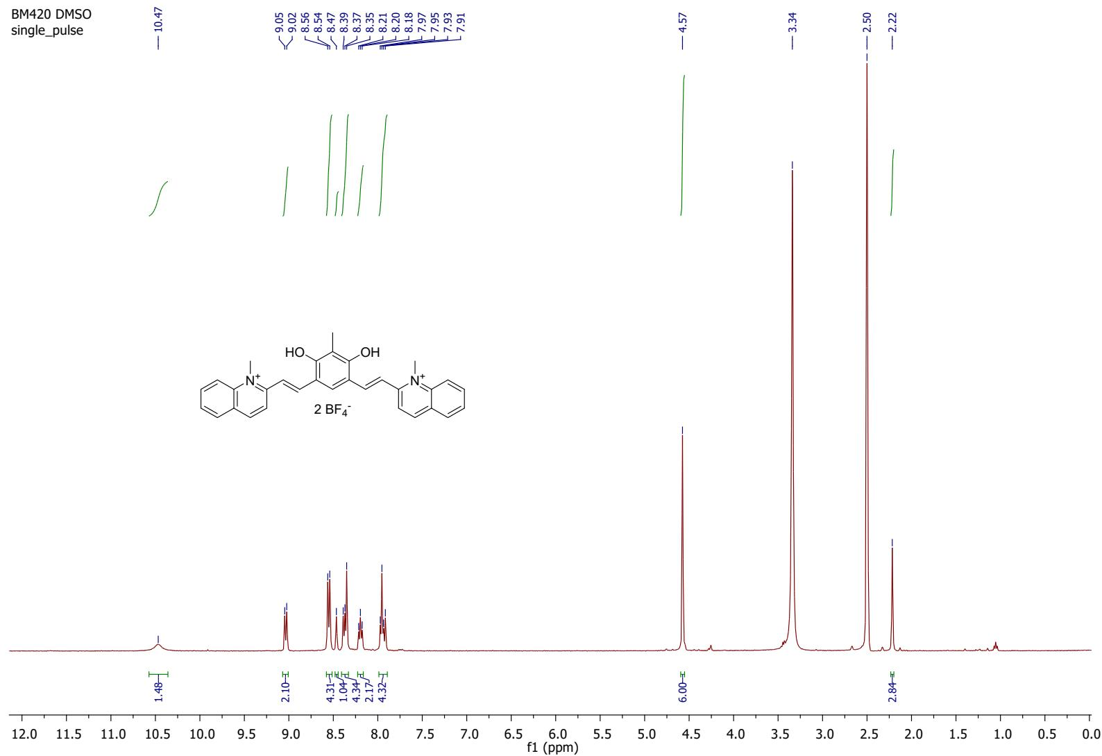
Figure S 32. <sup>1</sup>H NMR (400 MHz, DMSO-d<sub>6</sub>) of compound **4•2H<sub>2</sub><sup>+</sup>**.
