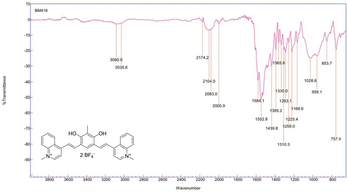
Figure S 66. Infrared spectrum of compound **5•2H<sup>+</sup>** (neat).
