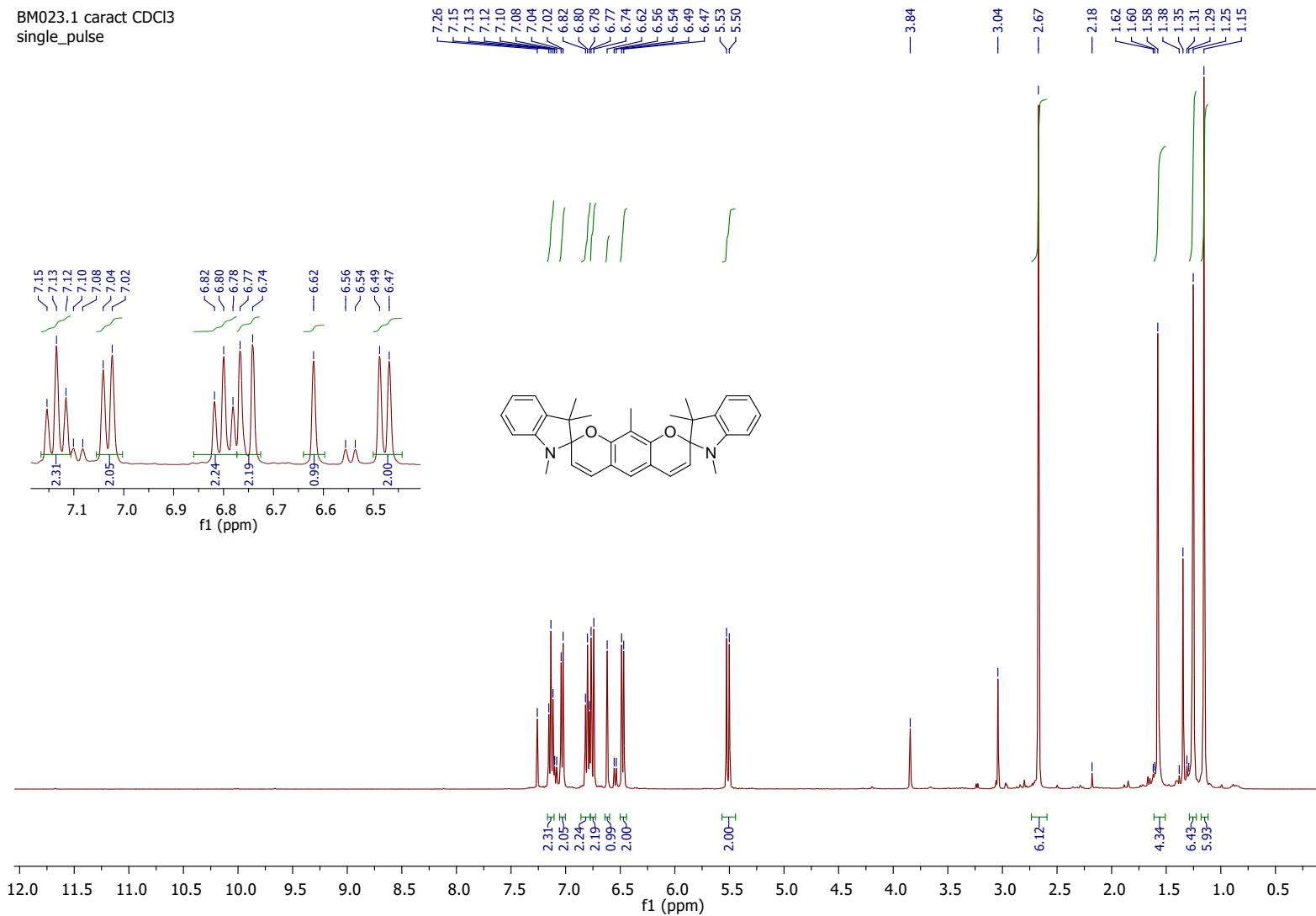
Figure S 13. <sup>1</sup>H NMR (400 MHz, CDCl<sub>3</sub>) of compound **dsp-1**.
