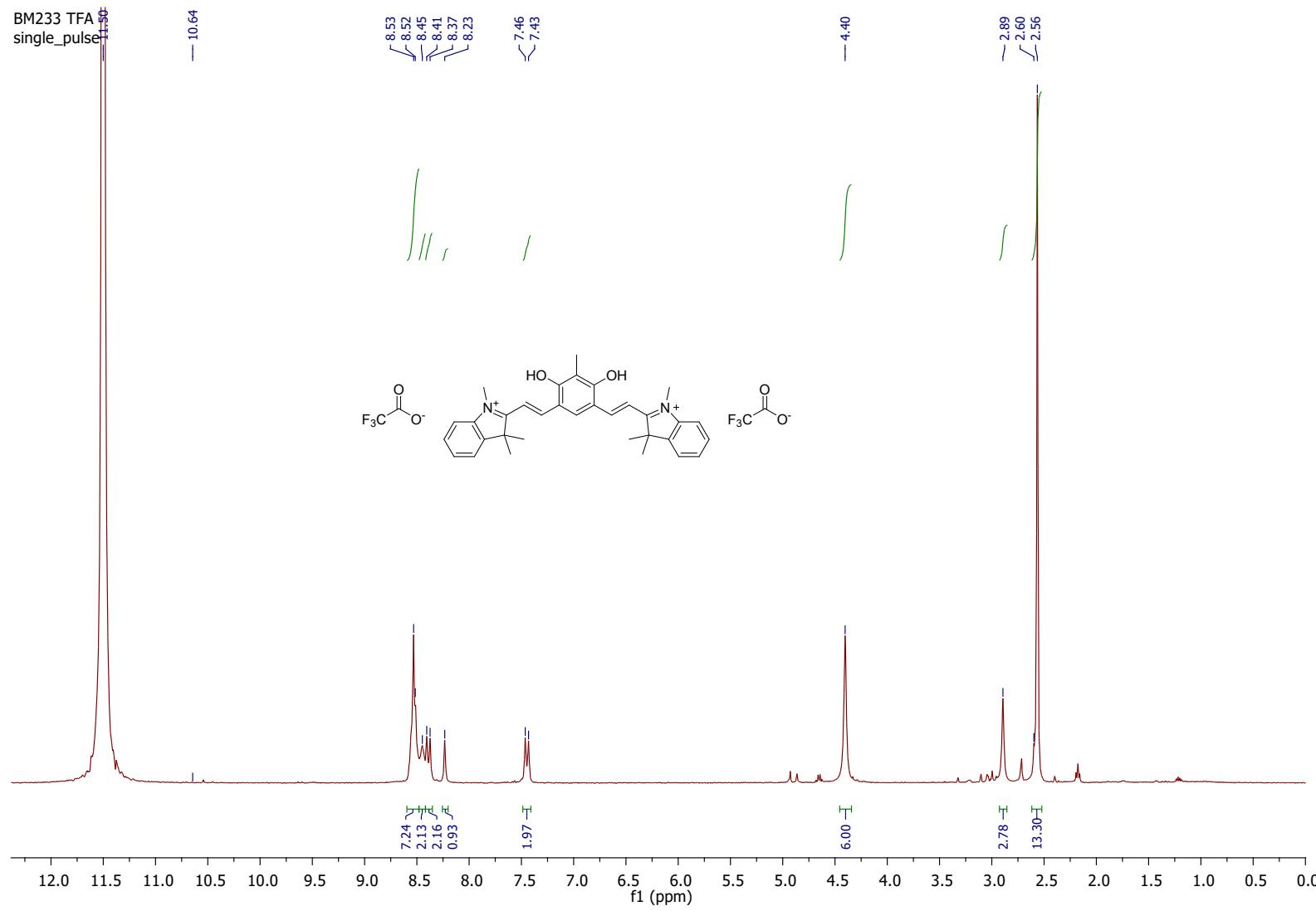
Figure S 18.  $^1\text{H}$  NMR (400 MHz, TFA-*d*) of compound **1•H<sup>2+</sup>**.
