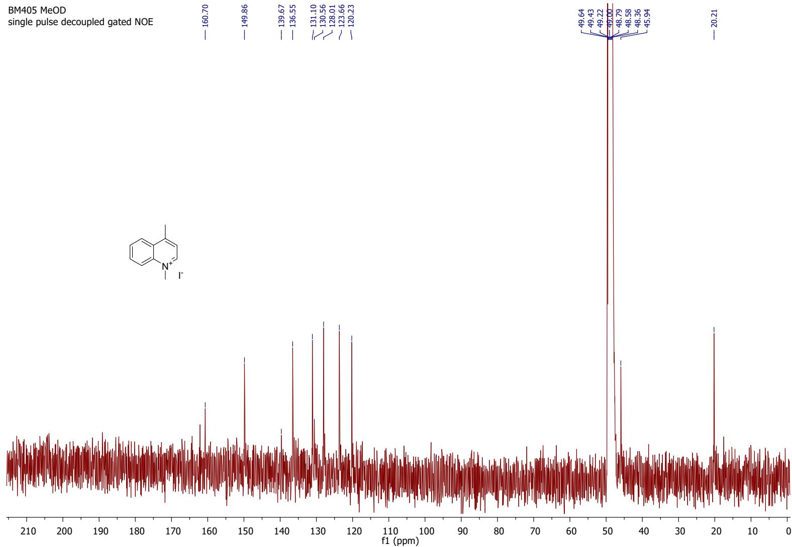
Figure S 12.  $^{13}\text{C}$  NMR (101 MHz,  $\text{CD}_3\text{OD}$ ) of compound 11.
