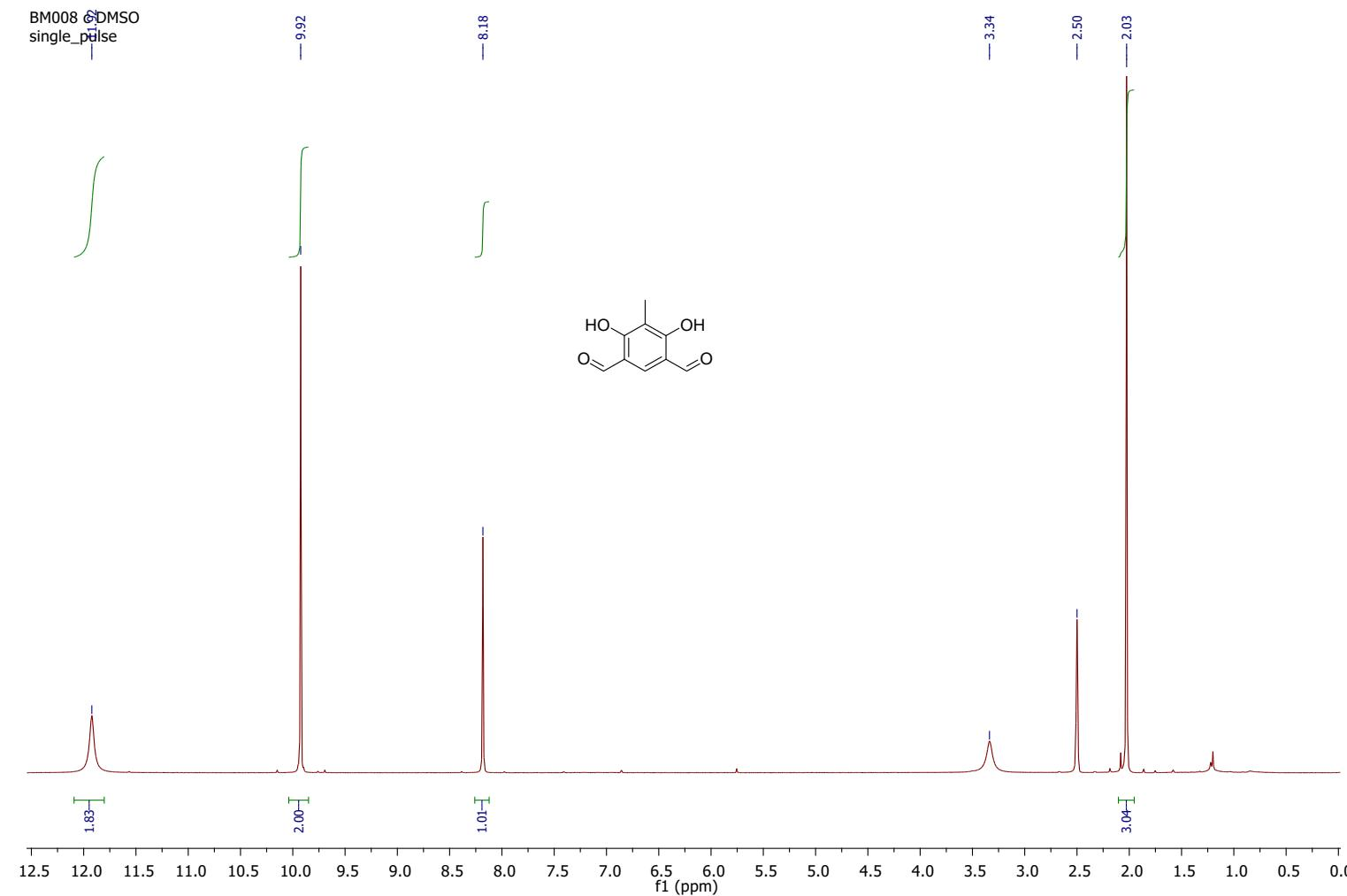
Figure S 1.  $^1\text{H}$  NMR (400 MHz,  $\text{DMSO}-d_6$ ) of compound 6.
