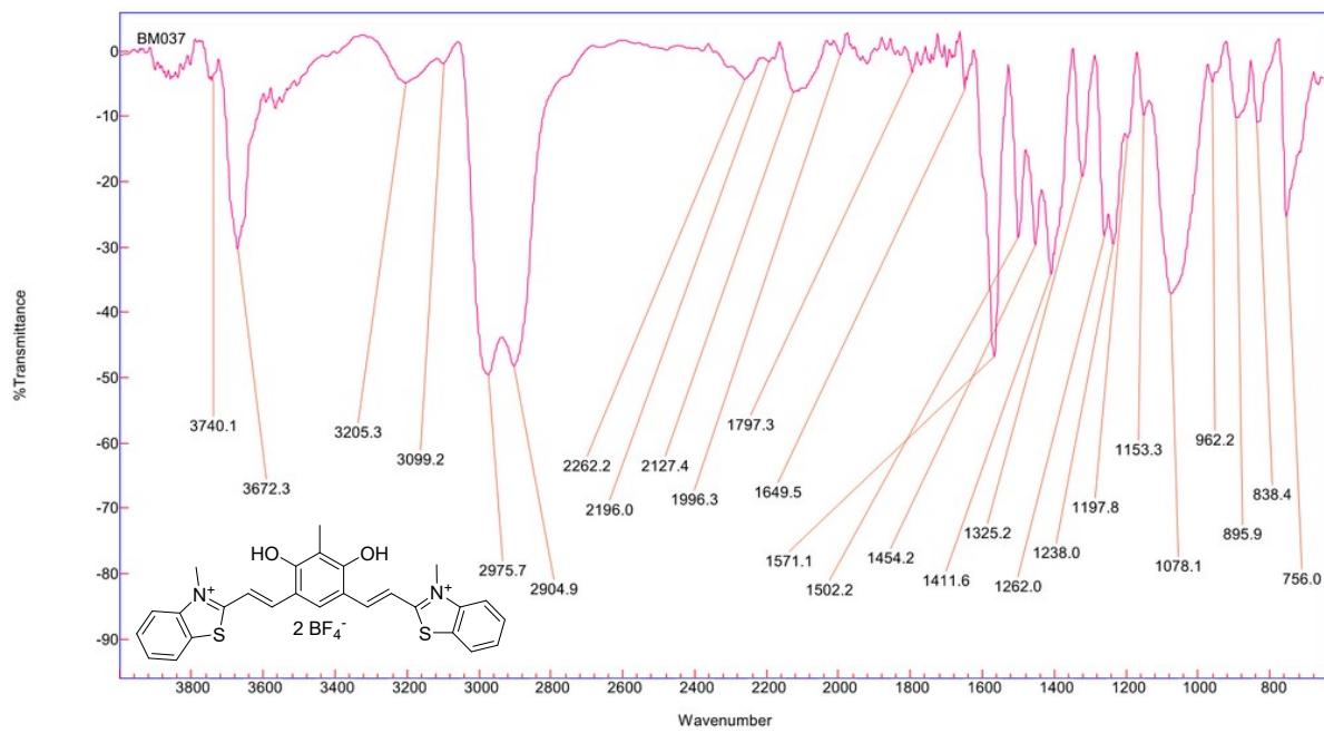
Figure S 64. Infrared spectrum of compound **3•2H<sup>2+</sup>** (neat).
