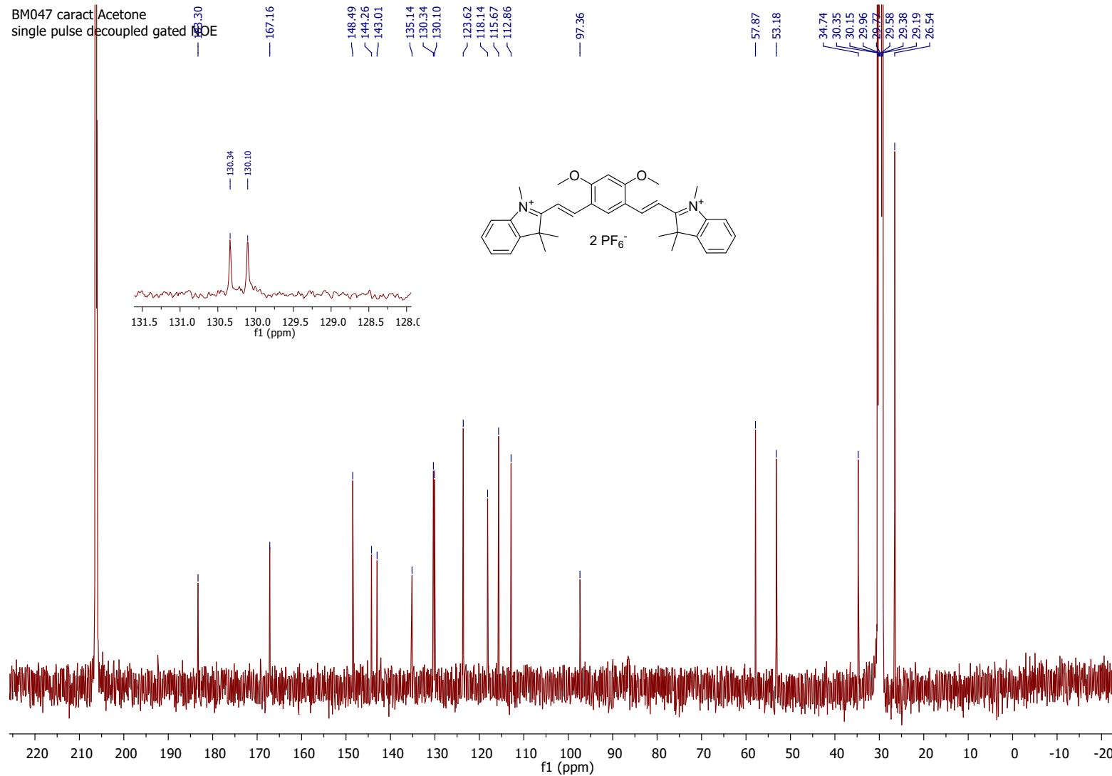
Figure S 46. <sup>13</sup>C NMR (101 MHz, Acetone-*d*<sub>6</sub>) of compound **1'**.
