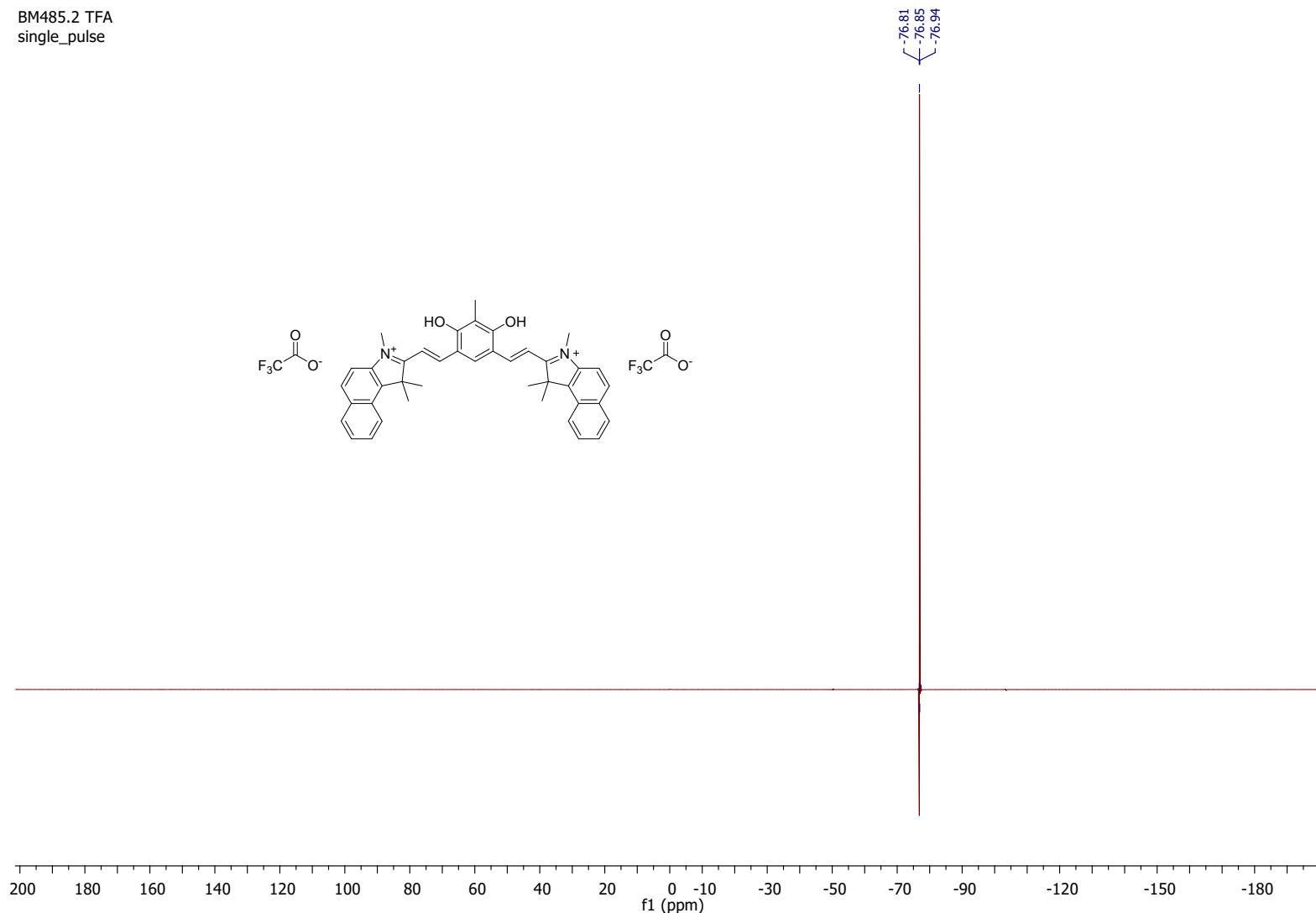
Figure S 27.  $^{19}\text{F}$  NMR (377 MHz, TFA-*d*) of compound **2•2H<sup>2+</sup>**.
