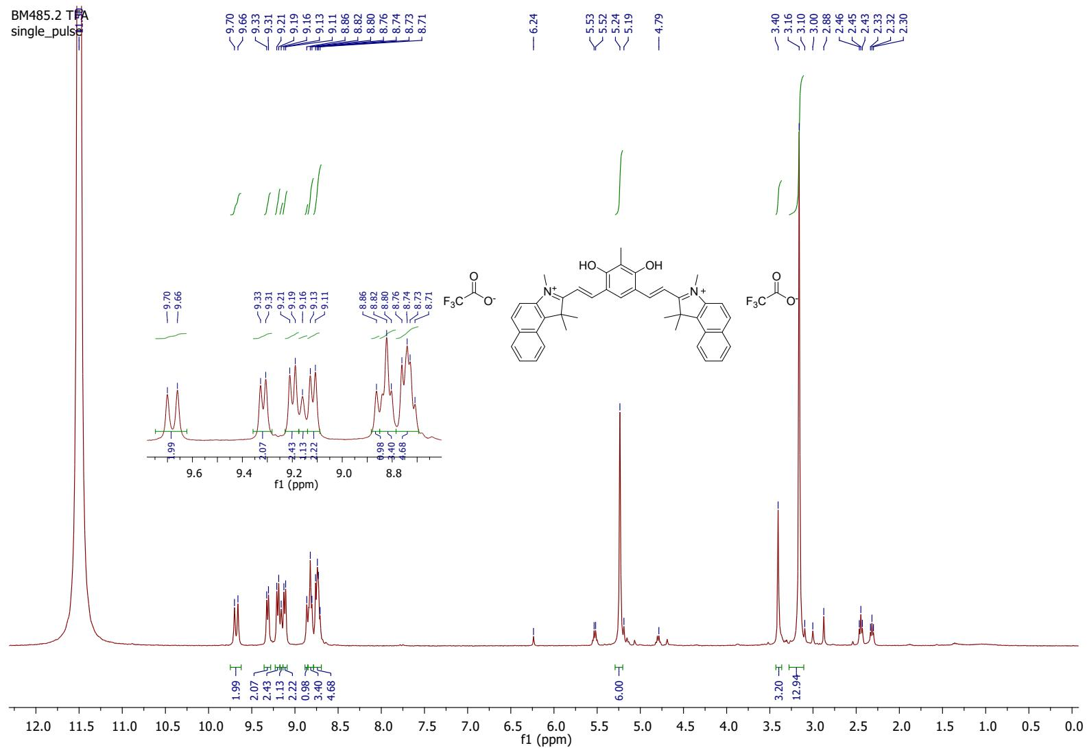
Figure S 26.  $^1\text{H}$  NMR (400 MHz, TFA-*d*) of compound **2** $\bullet$  $2\text{H}^{2+}$ .
