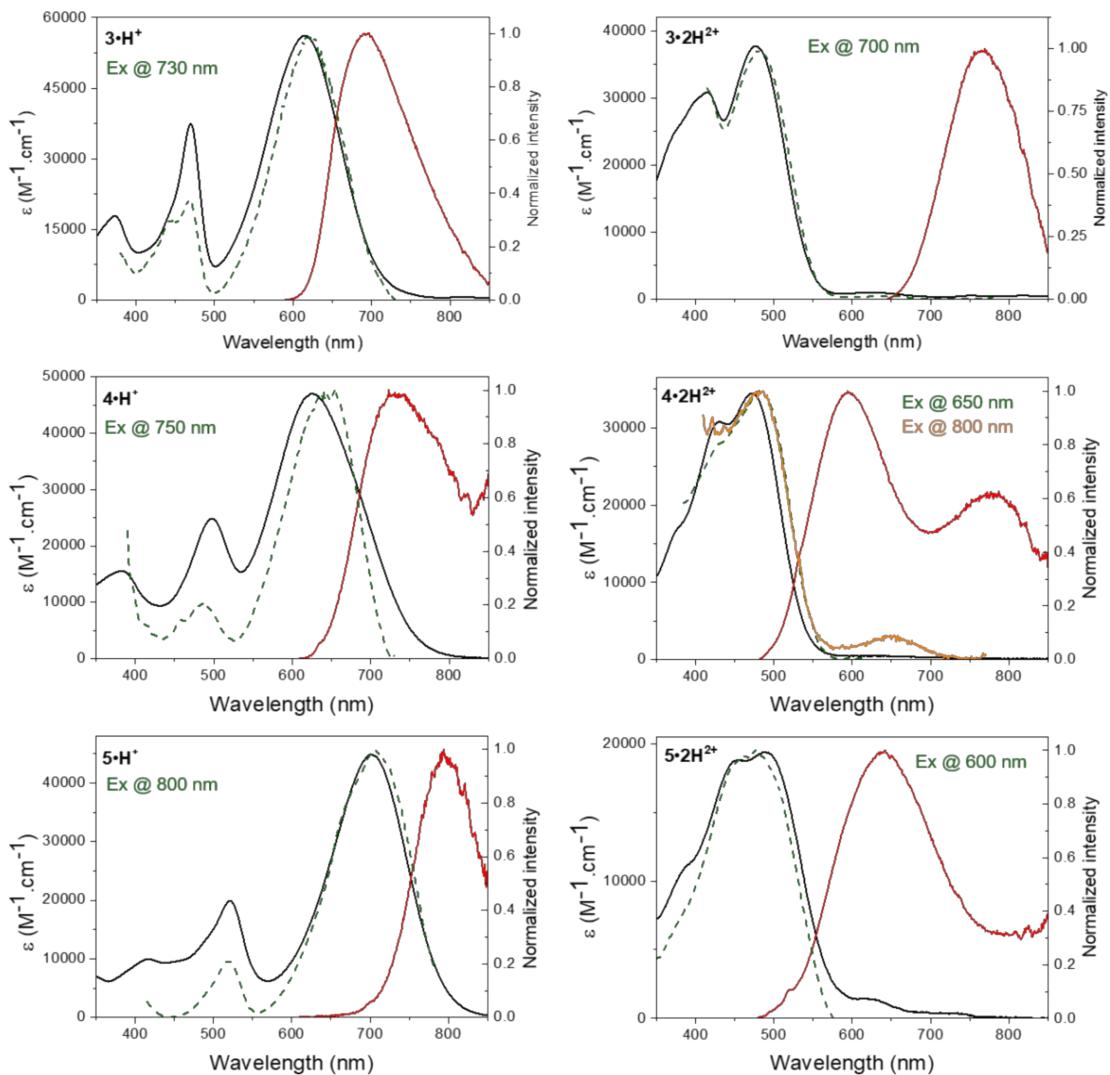
Figure S 79. Electronic absorption (black lines), normalized emission (red lines) and normalized excitation spectra (green dotted lines, with monitoring wavelength specified in green) of the emissive species **3–5** in MeOH. Note: for the emission of **4•2H<sup>2+</sup>**, the second band found between 700–850 nm is attributed to the presence of **4•H<sup>+</sup>** in solution, as revealed by the excitation spectrum recorded while monitoring the emission at 800 nm (orange curve).
