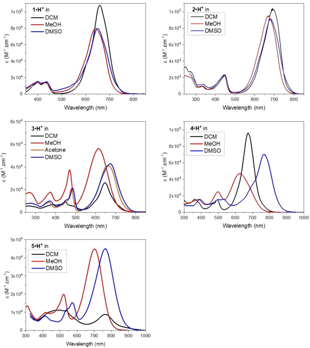
Figure S 72. UV-vis-NIR electronic absorption solvatochromism of cationic species recorded in various solvents. The cations **3**•H<sup>+</sup>, **4**•H<sup>+</sup> and **5**•H<sup>+</sup> were generated by dissolution of compounds **3**•2H<sup>2+</sup>, **4**•2H<sup>2+</sup> and **5**•2H<sup>2+</sup>, respectively.
