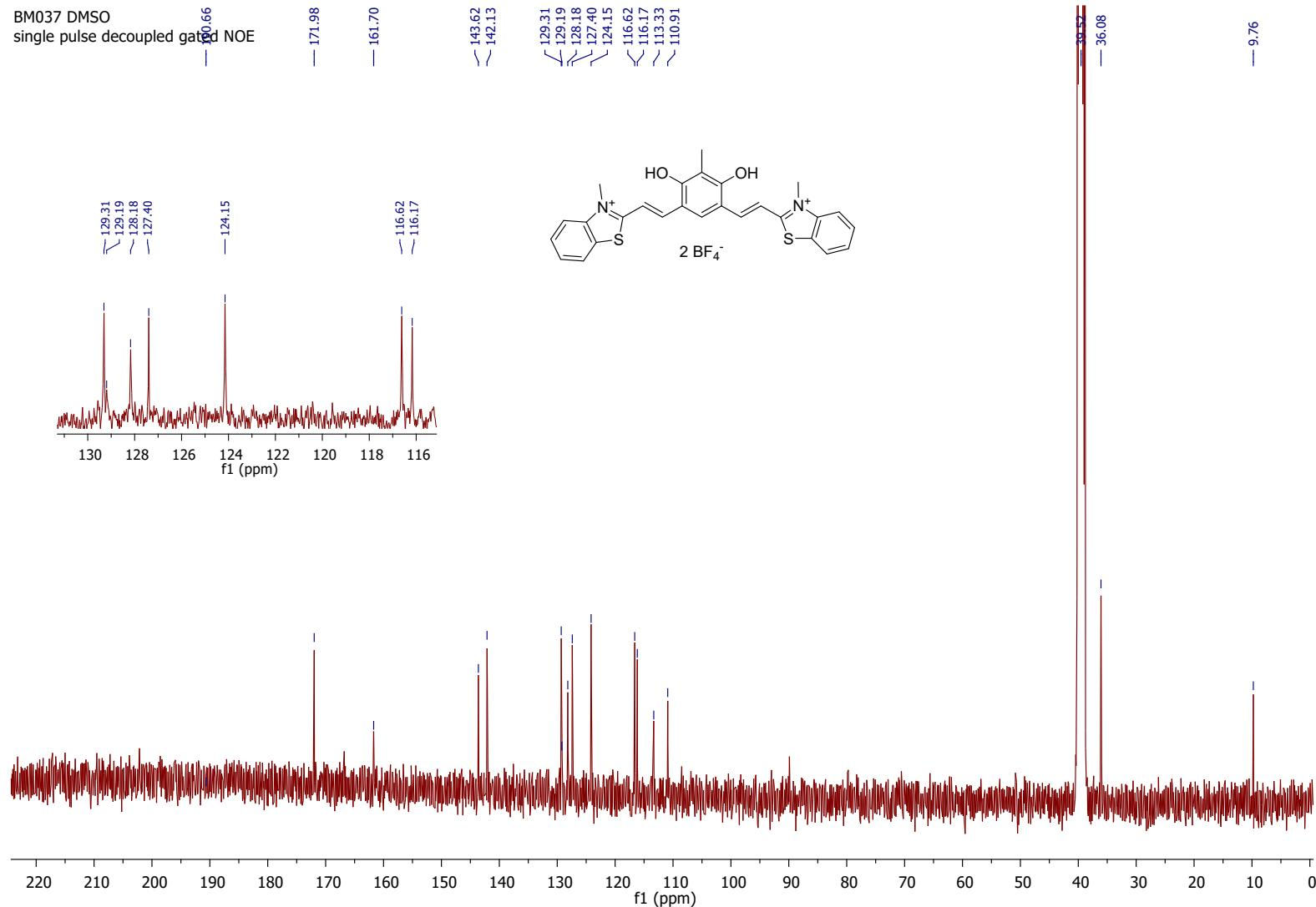
Figure S 31.  $^{13}\text{C}$  NMR (101 MHz,  $\text{DMSO}-d_6$ ) of compound  $3\bullet 2\text{H}^{2+}$ .
