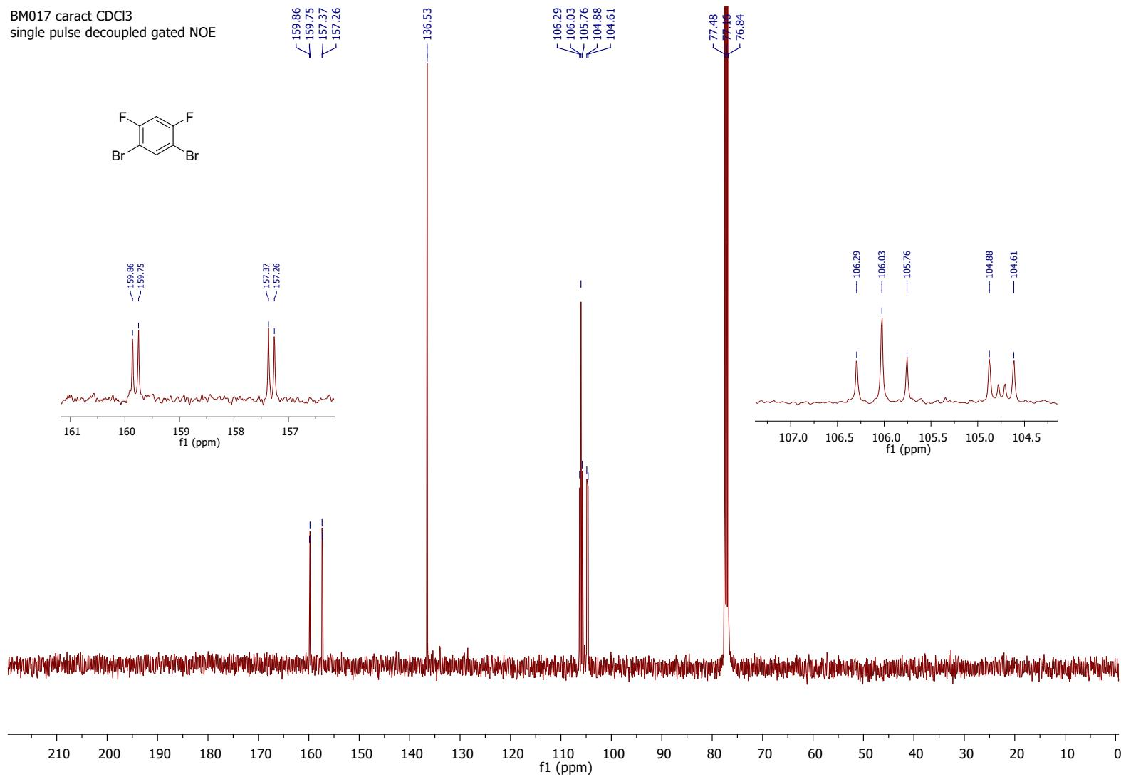
Figure S 40. <sup>13</sup>C NMR (101 MHz, CDCl<sub>3</sub>) of compound 13.
