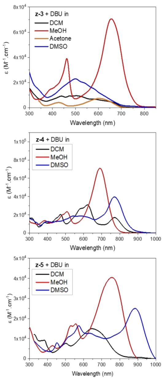
Figure S 73. UV-vis-NIR electronic absorption solvatochromism of zwitterionic species recorded in various solvents in the presence of DBU (0.1 M), generated *in situ* from **3•2H<sup>2+</sup>**, **4•2H<sup>2+</sup>** and **5•2H<sup>2+</sup>**.
