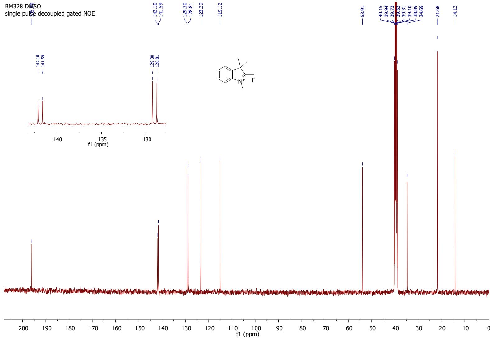
Figure S 4.  $^{13}\text{C}$  NMR (101 MHz,  $\text{DMSO}-d_6$ ) of compound 7.
