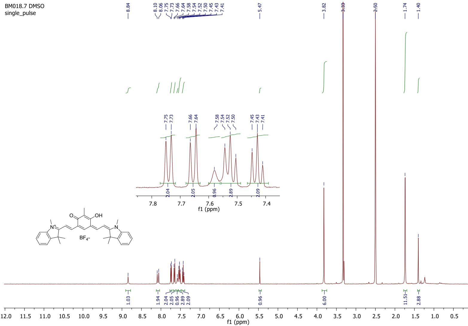
Figure S 15.  $^1\text{H}$  NMR (400 MHz,  $\text{DMSO}-d_6$ ) of compound **1•H<sup>+</sup>**.
