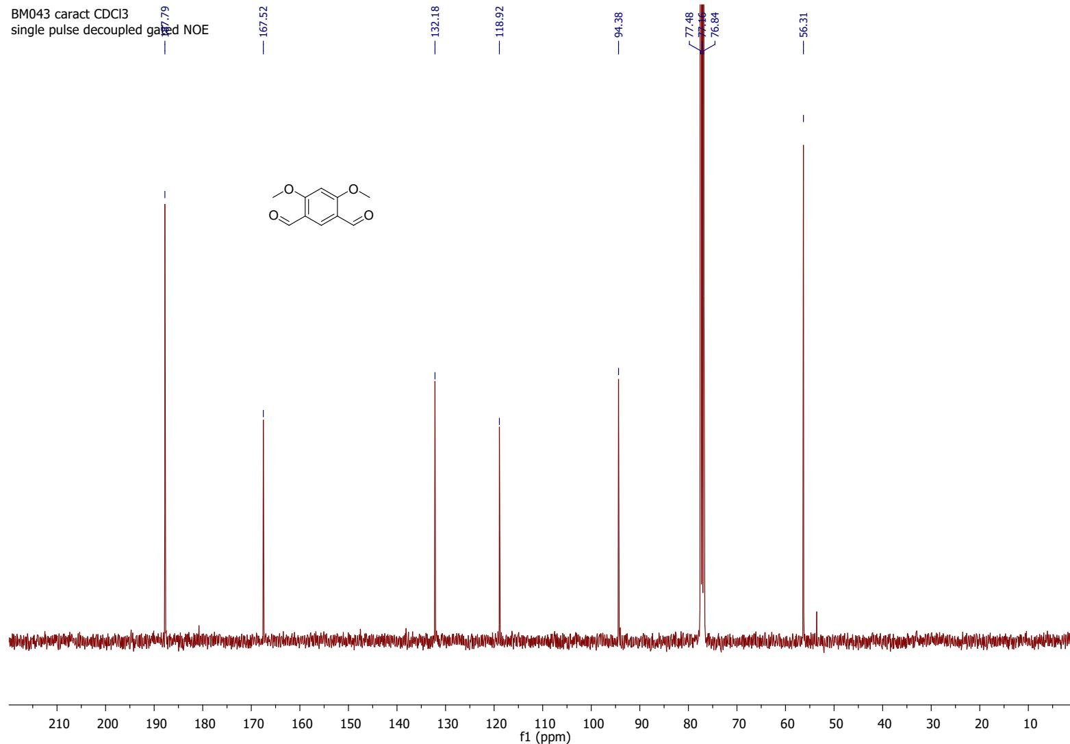
Figure S 44. <sup>13</sup>C NMR (101 MHz, CDCl<sub>3</sub>) of compound **12**.
