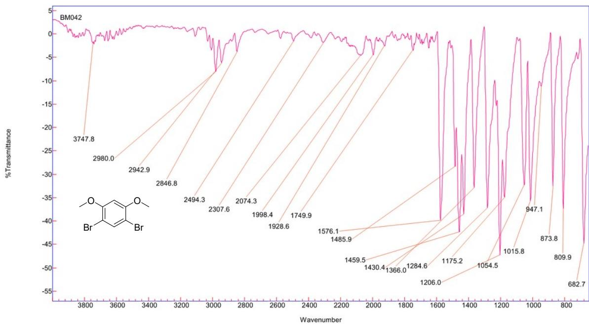
Figure S 68. Infrared spectrum of compound **14** (neat).
