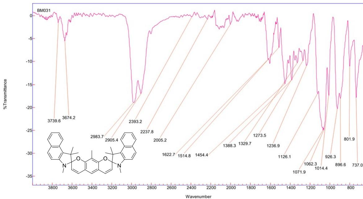
Figure S 62. Infrared spectrum of compound **dsp-2** (neat).
