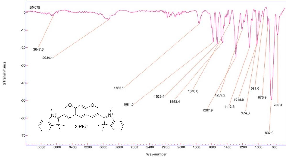
Figure S 70. Infrared spectrum of compound 1' (neat).
