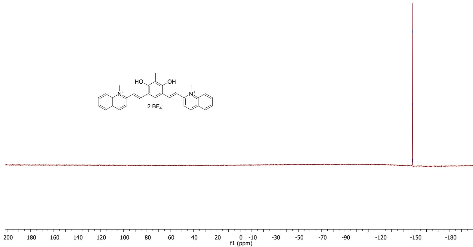
Figure S 33.  ${}^{19}\text{F}$  NMR (377 MHz,  $\text{DMSO}-d_6$ ) of compound  $4\bullet 2\text{H}^{2+}$ .
