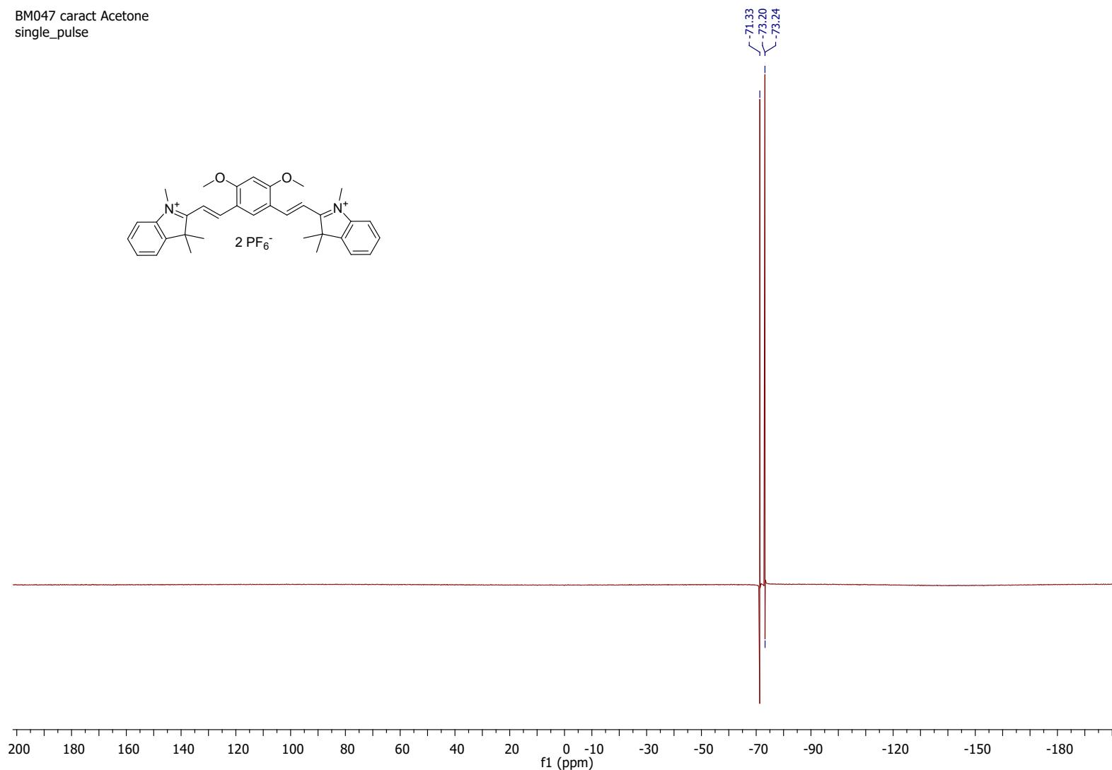
Figure S 47. <sup>19</sup>F NMR (101 MHz, Acetone-*d*<sub>6</sub>) of compound **1**.
