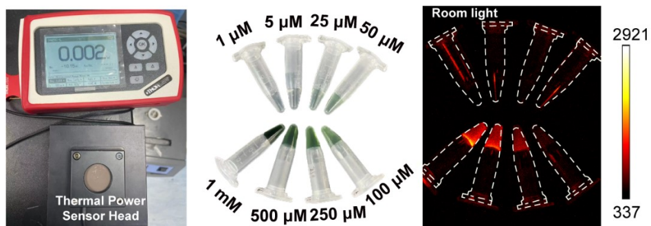
Supplementary Figure 3. TPA-TQT NIR-II imaging excited by LED room light without other excitation light sources. (1000 nm LP, 1000 ms, 0.35 \text{ mW cm}^{-2} ).
