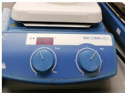
**Figure S20** Standard magnetic stirrer hot plate used for Hg drop test, with vigorous stirring. The temperature of the probe (picture not shown) was set to the desired reaction temperature (*i.e.* ‘bath temperature’), as is typical practice. Through control experiments on similar equipment, we estimate the temperature difference inside the reaction flask to be ( $\pm 2$  °C). This information is given in the revised SI document.
