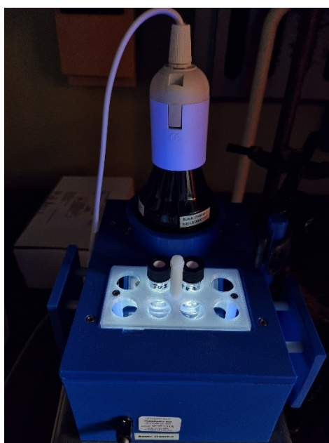
Figure S1. The photocatalytic setups with one lamp (left) and with two lamps (right).
