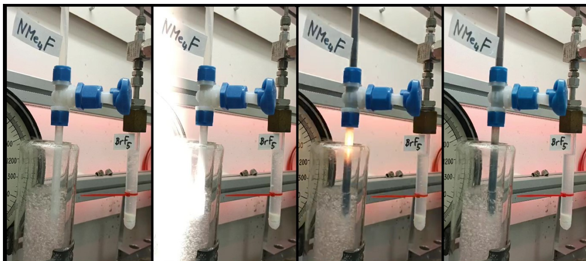
Figure S1. Four consecutive frames of a video of the reaction of [\text{NMe}_4]\text{F} with \text{BrF}_5 . The right vessel contains [\text{NMe}_4]\text{F} and is cooled in a Weinhold vessel filled with liquid nitrogen. On the right side is the vessel containing \text{BrF}_5 , which is connected to the left vessel via the Schlenk line. As soon as \text{BrF}_5 starts to condense in the left reaction vessel, it starts reacting. A bright flash (second frame) followed by an orange-yellow flame shooting upwards through the vessel (third frame) can be seen. After the reaction, the vessel is still intact and only covered by a dense layer of soot (fourth frame) that can be wiped off again.
