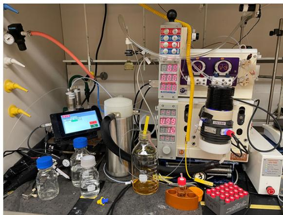
**Figure SI.9. Scale-up experiments in a Vaportec photoreactor.**
