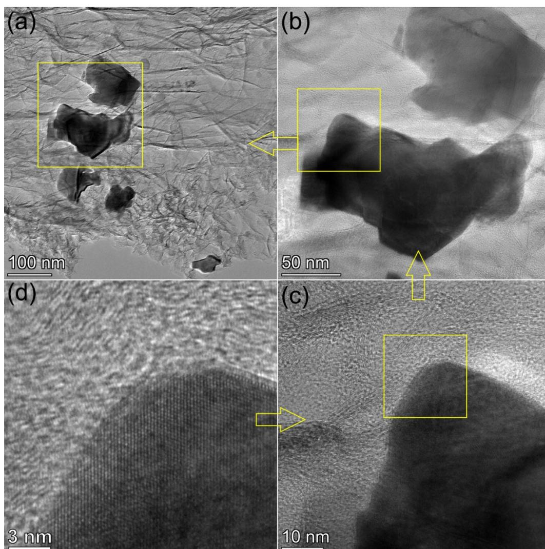
**Figure S4:** TEM images at different magnifications of Ni@rGO 900 material.
