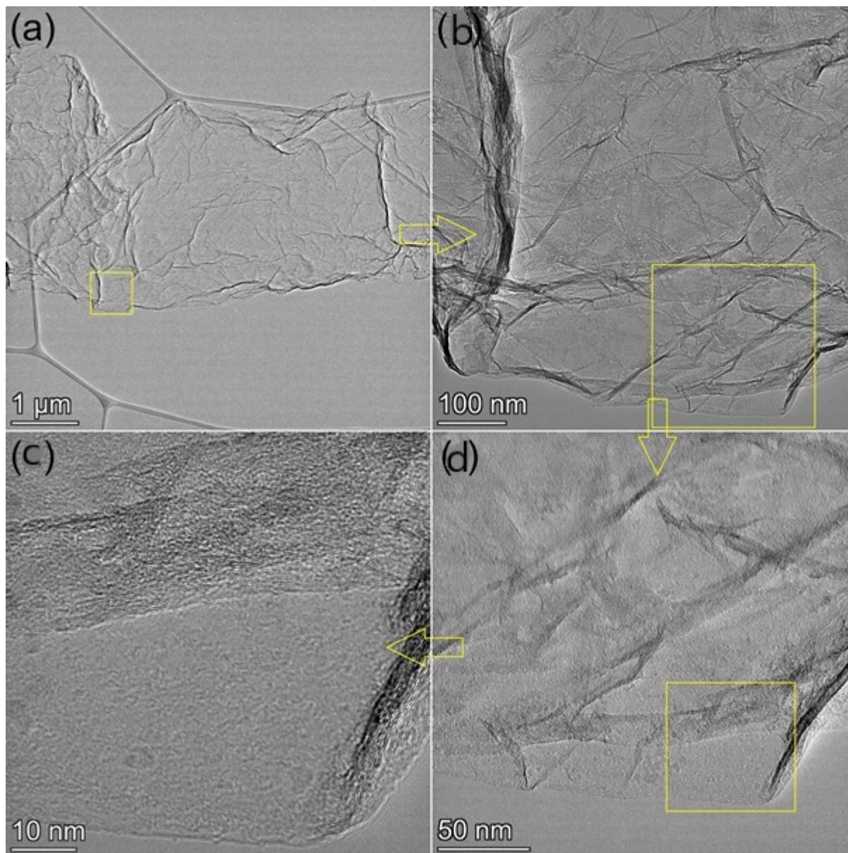
**Figure S2:** TEM images at different magnifications of Ni@rGO material.
