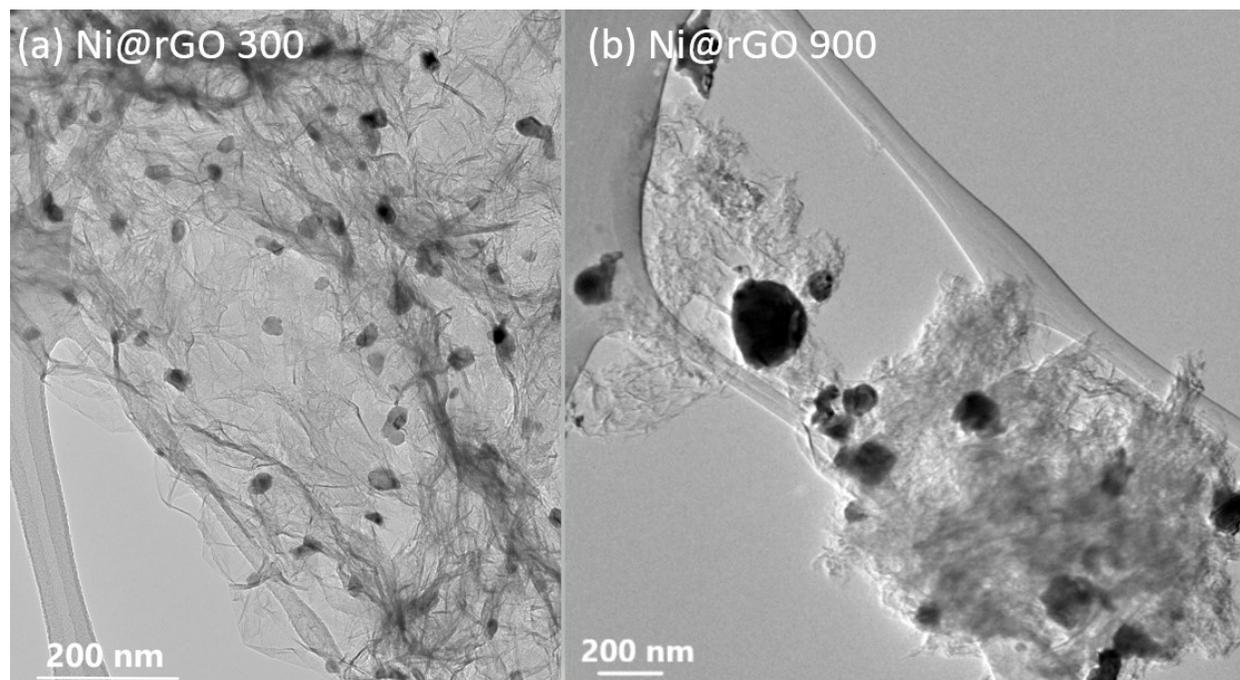
**Figure S1:** The TEM images of a) Ni@rGO 300 and b) Ni@rGO 900.
