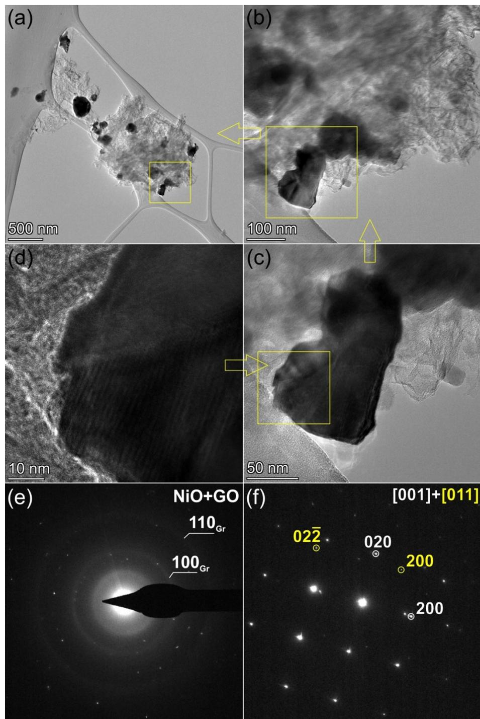
**Figure S5:** (a-d) A series of bright-field TEM images of Ni@rGO 900 material taken at different magnifications. (e) The electron diffraction, obtained from the entire region shown on (a). (f) The electron diffraction from an individual nanoparticle. The ED image (f) is indexed in the NiO cubic lattice.
