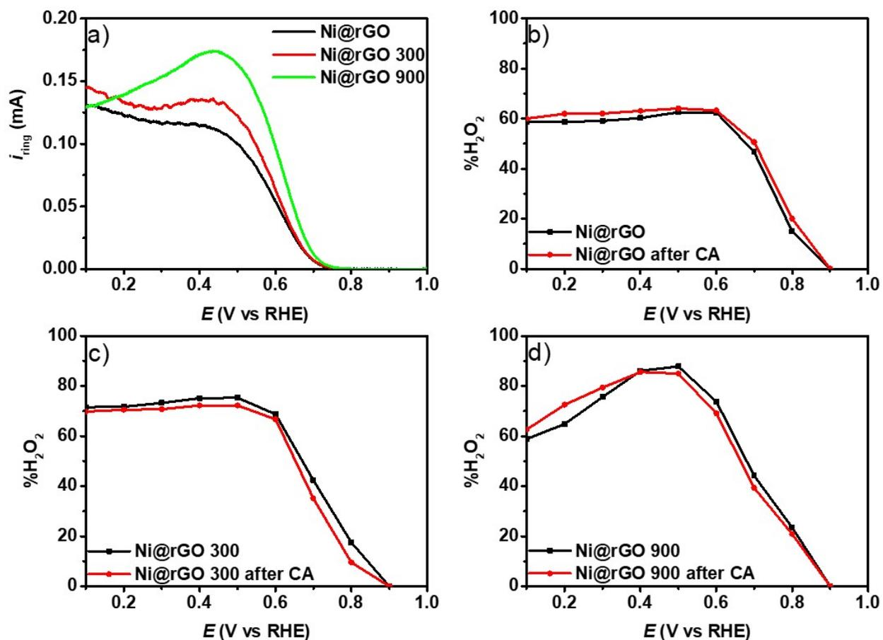
**Figure S11:** a) Current on the ring part of RRDE (at constant  $E = 1.3$  V vs RHE) during the ORR selectivity study and the selectivity after the two-hour CA stability measurement for b) Ni@rGO c) Ni@rGO 300 and d) Ni@rGO 900 (green) in O<sub>2</sub> saturated 0.1 M KOH.
