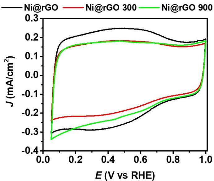
**Figure S10:** The CV of Ni@rGO (black), Ni@rGO 300 (red) and Ni@rGO (green) performed in Ar saturated 0.1 M KOH solution at a scan rate of 20 mV and 1600 rpm rotation speed.
