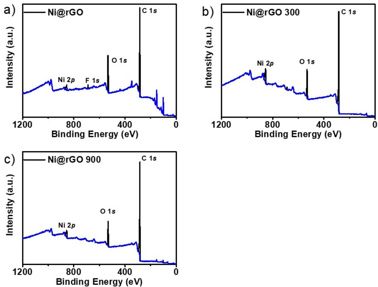
**Figure S7:** XPS survey spectra of a) Ni@rGO, b) Ni@rGO 300 and c) Ni@rGO 900 materials.
