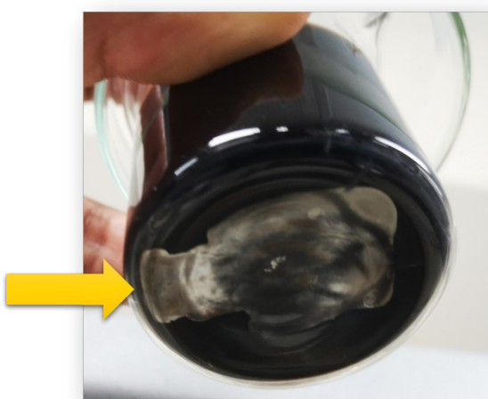
Figure S1. Photograph showing the deposition of Ni particles after the galvanic replacement by Ru on the nickel foam (NF) surface after 24 h immersion in RuCl 3 solution.
