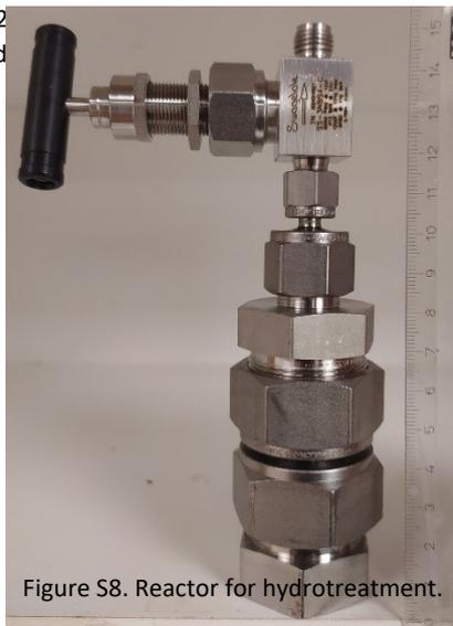
Figure S8. Reactor for hydrotreatment.
