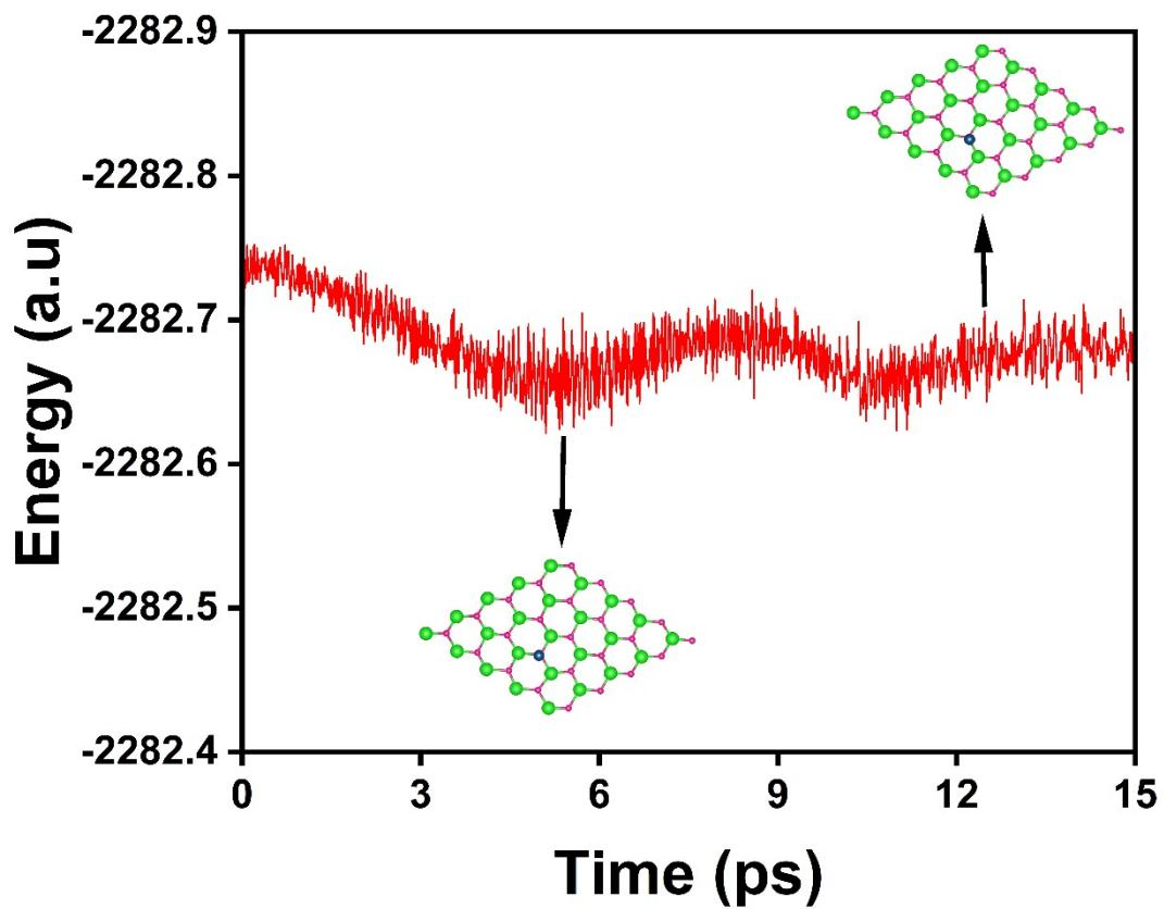
**Fig. S5:** Variation of energy versus the AIMD simulation time for Ni@GaN for 15 ps at 600K. The insets are the top views of snapshots of configurations at 5 and 12 ps.
