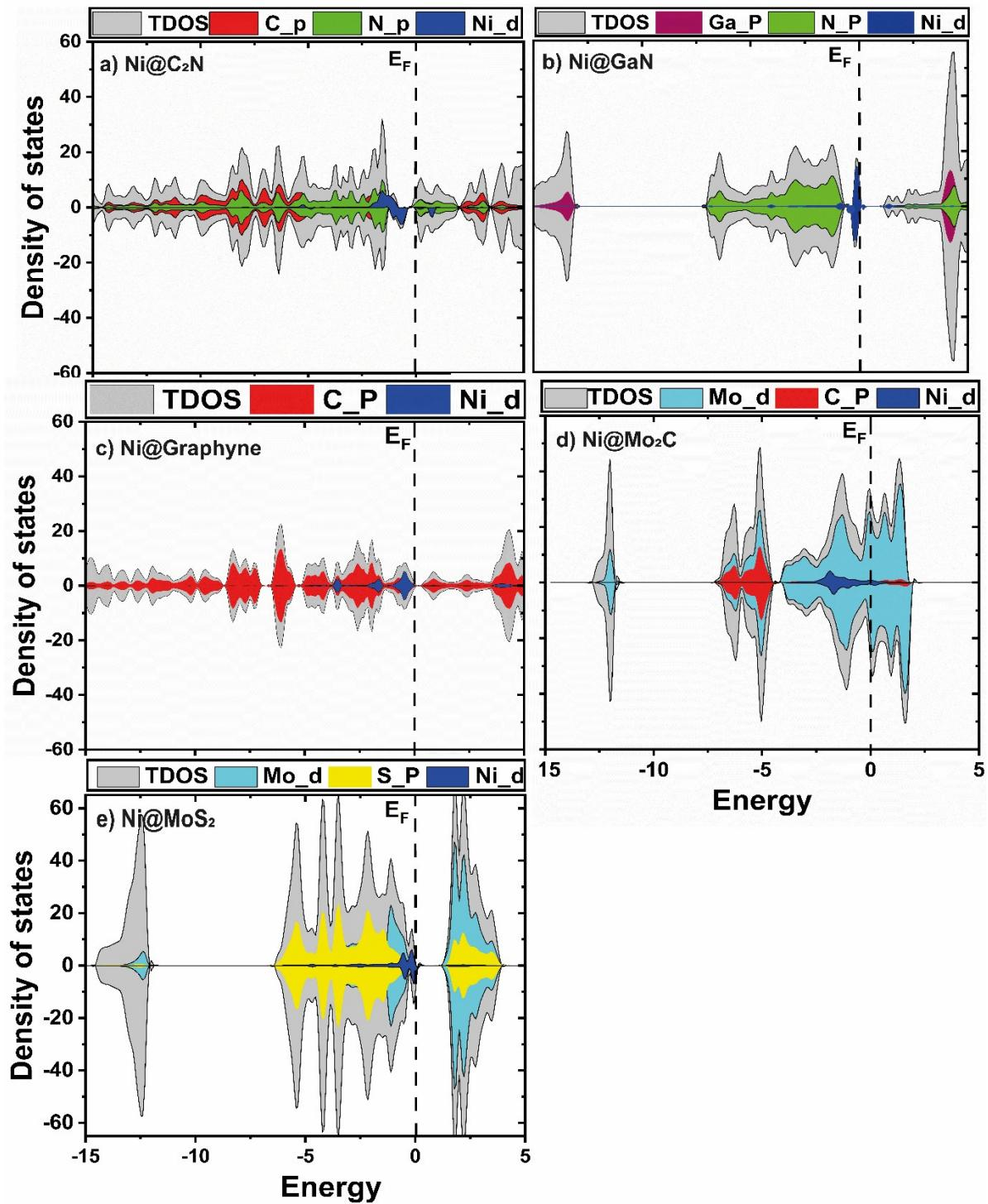
**Fig. S1.** Spin polarized orbital projected density of states (oPDOS) of Ni SACs supported on different monolayers. Colour codes for the orbital contributions are given in the plots. Fermi-level is set to zero.
