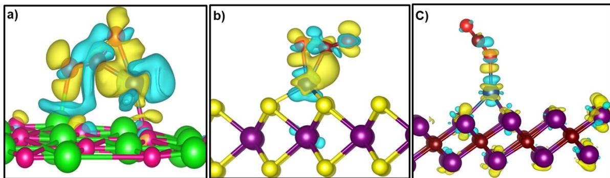
**Fig. S3:** Charge density difference plots of  $\text{CO}_2$  adsorbed on (a)  $\text{Ni@GaN}$  (b)  $\text{Ni@MoS}_2$  (c)  $\text{Ni@Mo}_2\text{C}$  catalysts. Yellow and cyan represents charge accumulation and depletion, respectively. The isosurface value was set to  $0.002 \text{ e}/\text{bohr}^3$ .
