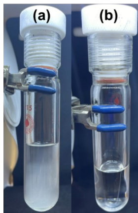
Figure S3: Fructose solubility studies in the absence of a catalyst: (a) 2 mL of a 25 wt% aqueous solution of fructose and 8 mL acetone and (b) 2 mL of a 25 wt% aqueous solution of fructose and 5 mL acetone.
